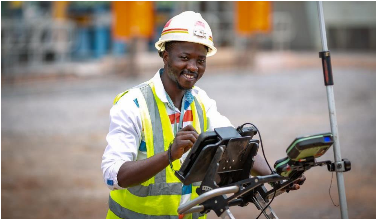
Surveyor Lumbu Ghislain Pansemoya using ground-penetrating radar to locate underground piping and cabling.
