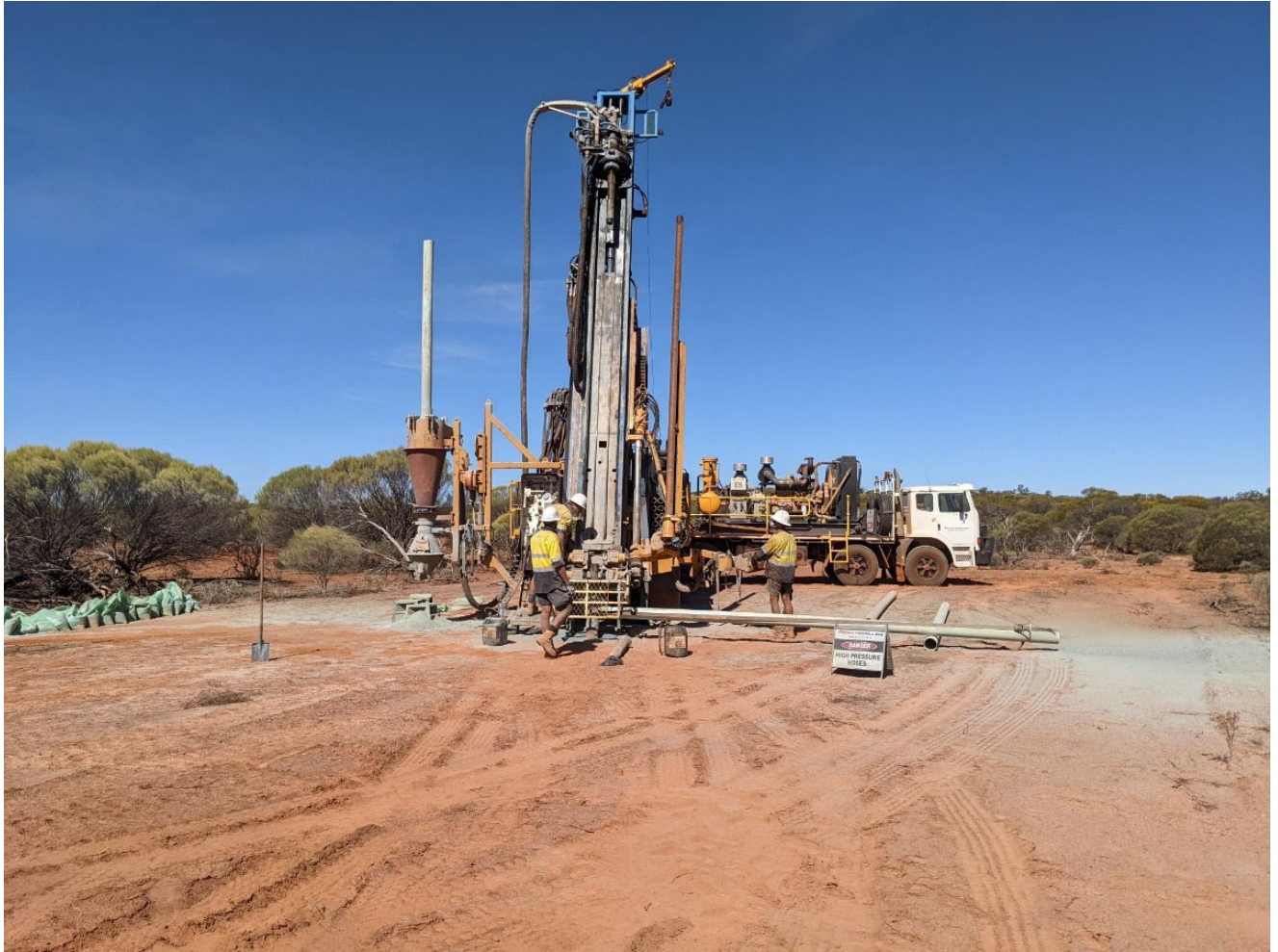
Figure 1: Reverse Circulation Rig on site drilling 2022 collar for EM platform hole at Tulloch.
