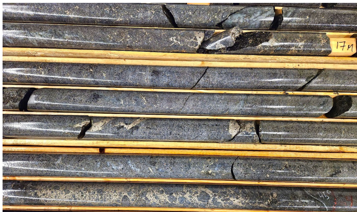
Figure 1: New drill core from VW-23-03 showing partial section from 15 metres to 24 metres. Interval of visual sulfides with pyrrhotite and visually identified interstitial chalcopyrite and pentlandite within the pyrrhotite showing disseminated to blotchy and net-texture. Bottom contact at 45 degrees.
