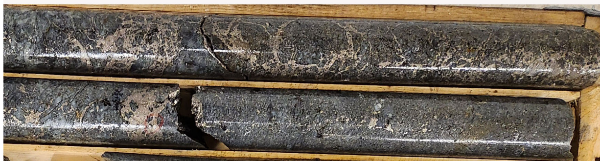
Figure 2: Drill hole VW-23-03 section from 1 to 4 meters downhole showing disseminated coarse patches of pyrrhotite with visually identified interspersed chalcopyrite and pentlandite within pyrrhotite.
