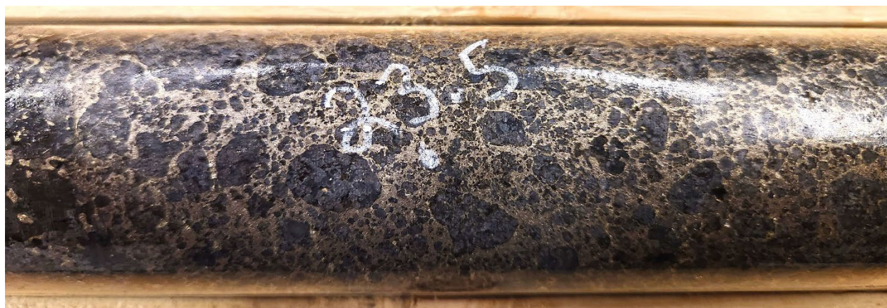
Figure 3: Close up core photo from VW-23-03 at 23.4 metres down hole showing sulfide matrix net-texture.
