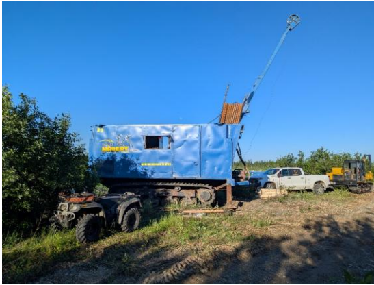
Figure 2. Diamond drill operating at the Estrades Project.
