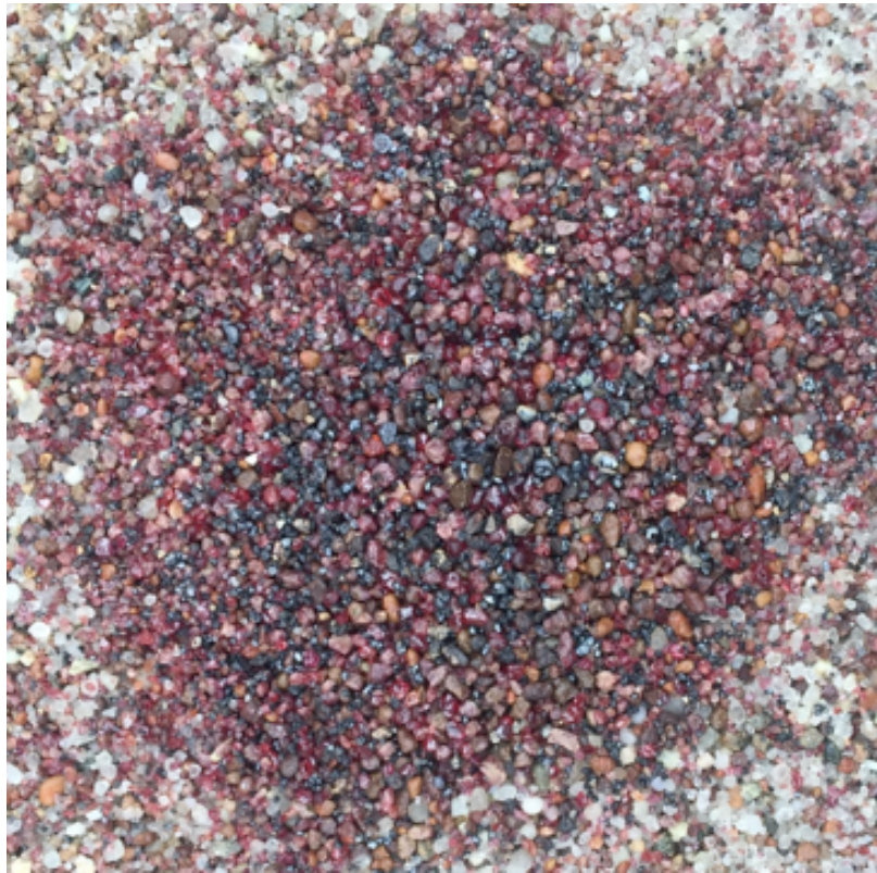
Garnets are so abundant within the concentrate, that approx. 40% of the concentrate retrieved is composed of garnets
