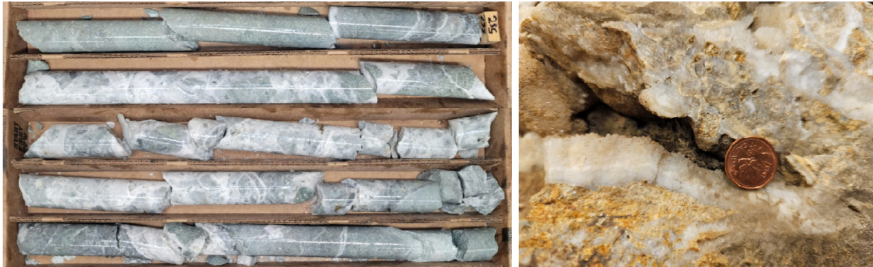
Figure 1. Photo of drill core from FHS24-03 and outcrop sample showing the vein and high-level textures expected above boiling zone.
