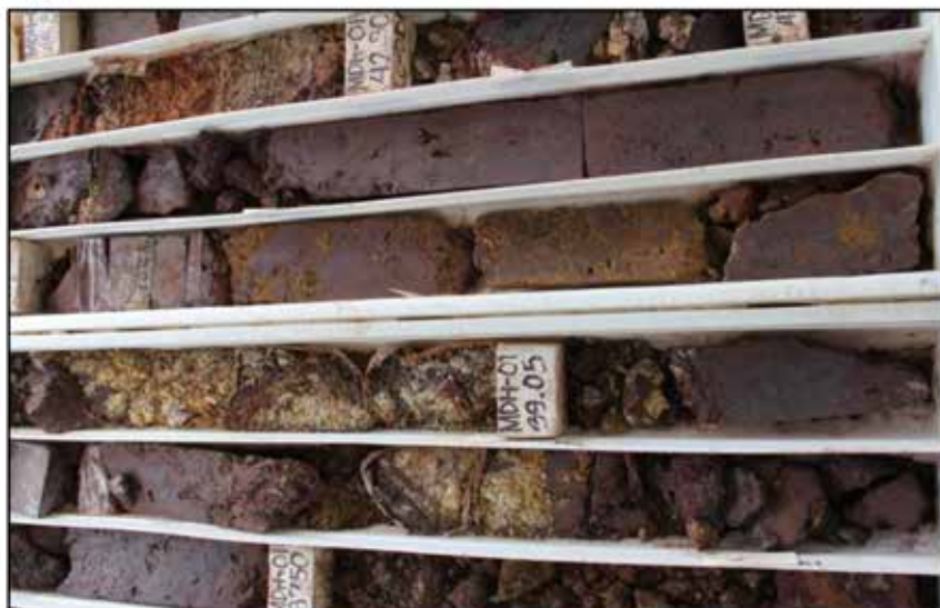
Photograph 4: Oxidised hematitic mineralisation after massive magnetite skarn with intervals of deeply weathered calc-silicate hornfels or skarn. 63 mm HQ core, MDH-01.
