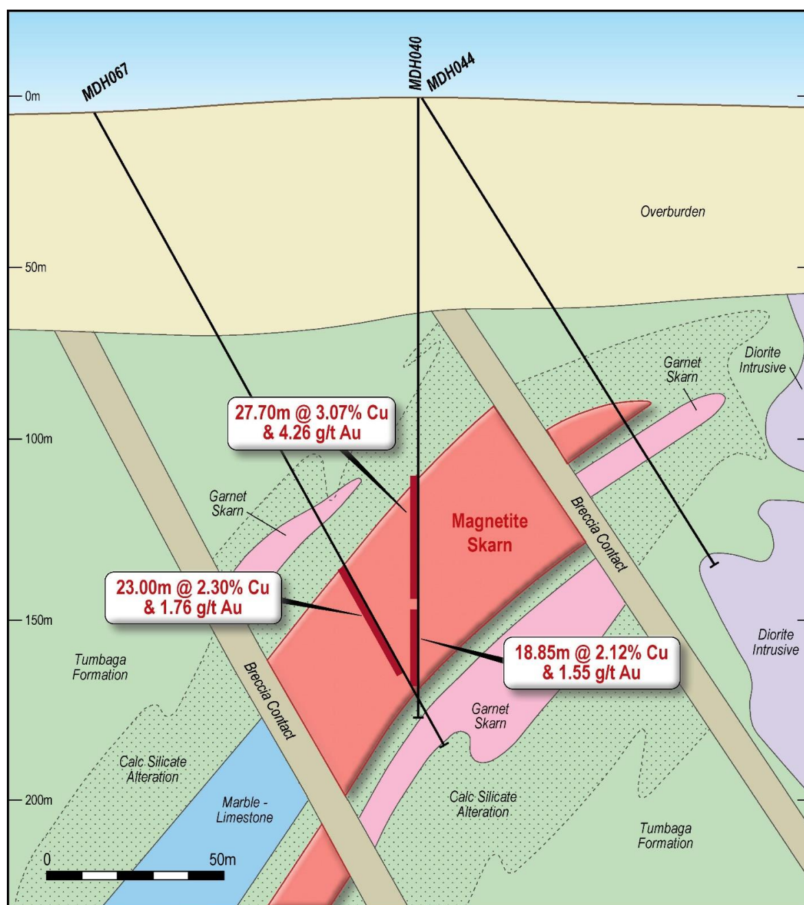
Figure 7. Intercept MDH067 through magnetite skarn down dip of MDH040.
