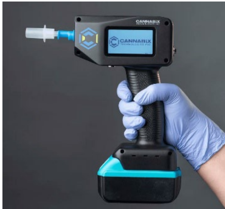
Cannabix Marijuana Breath Test hardware including Breath Collection Unit (BCU) and Breath Cartridge (BC) technologies for use in laboratory-based analysis
