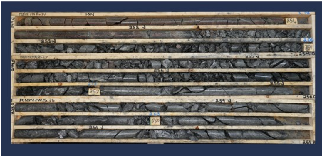
Figure 2: PLN24-144 (line 2820S): Basement wedge hosted graphitic fault
