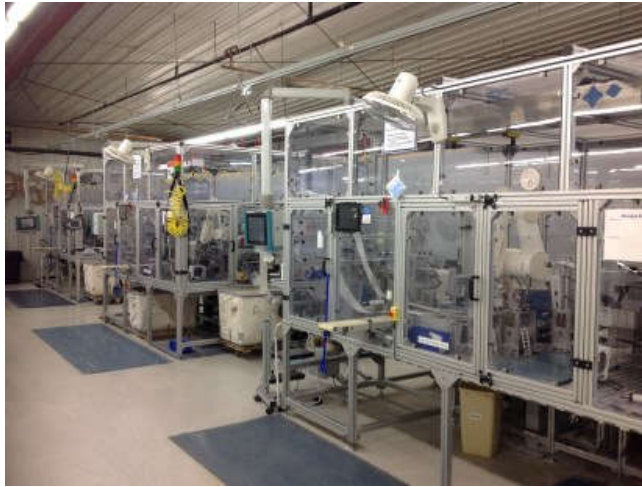
Above: Custom designed, robotic, automated production cells. These systems were designed and fabricated onsite by SDP.
