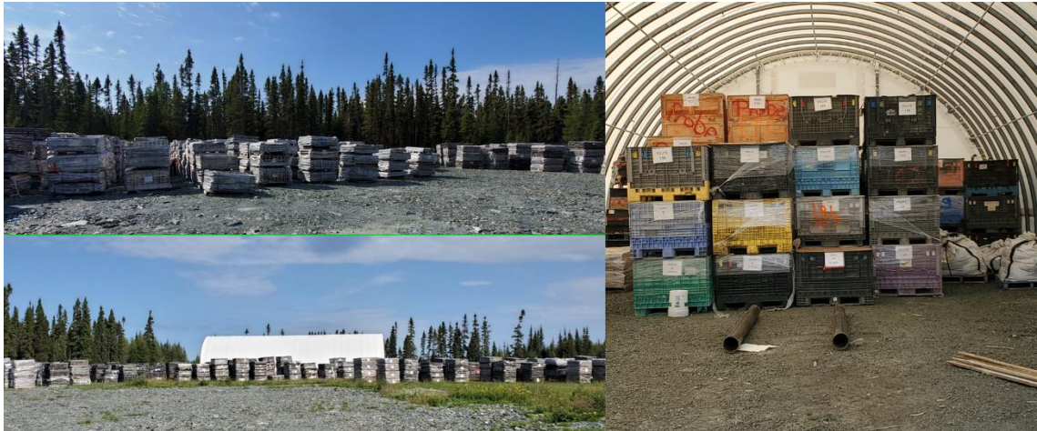
Figure 12.1 – Core and Pulp Storage
