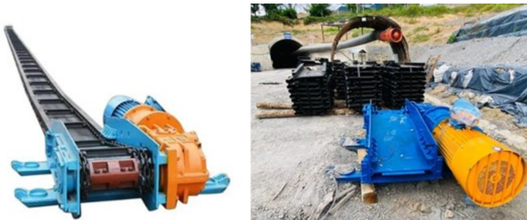
Figure 1. Panzer located onsite ready to be implemented
