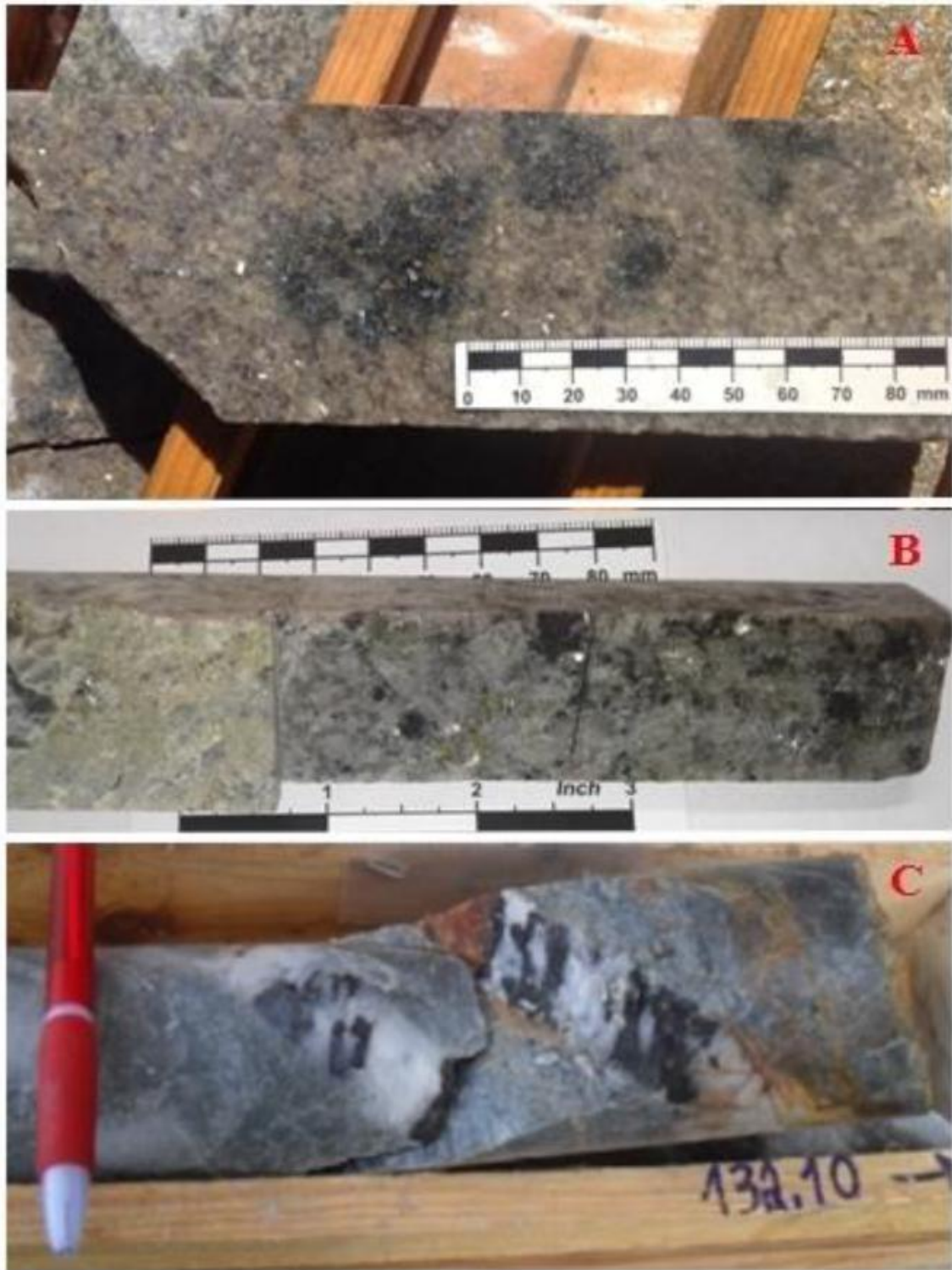
Figure 8-2:Core photographs showing the distinct types of mineralization of the Santa Helena Breccia- A) fine-grained wolframite and scheelite disseminated, B) Medium- to coarse-grained wolframite hosted in the siliceous cement, C) Coarse-grained wolframite occurring in late quartz veins.
