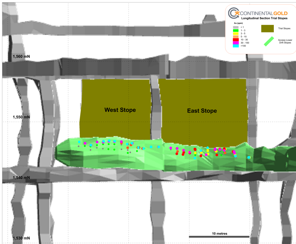
Figure 2 – Long section (at elevation of 1,550 metres) and sectional views of the completed East and West stopes and lower access drift.
