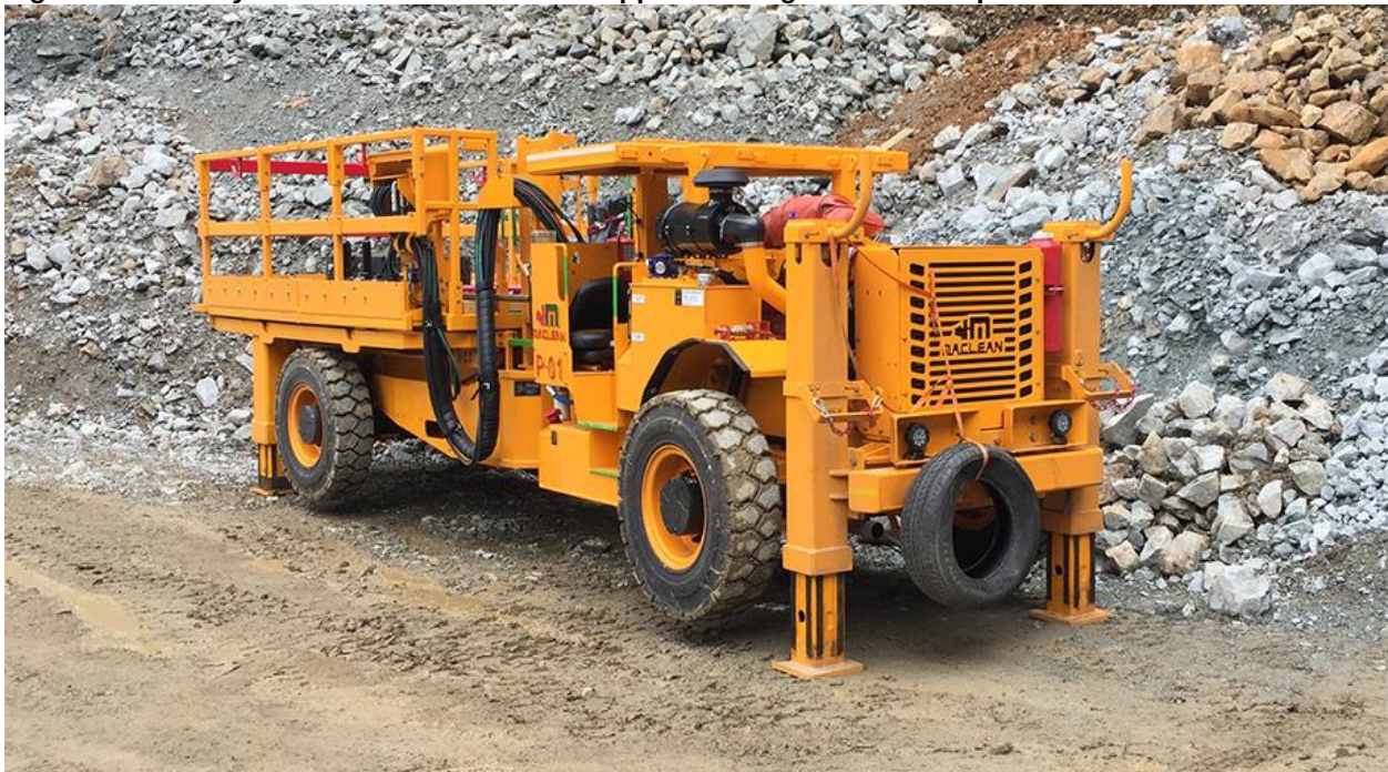
Figure 5: Recently-delivered Scissor Lift to Support Underground Development
