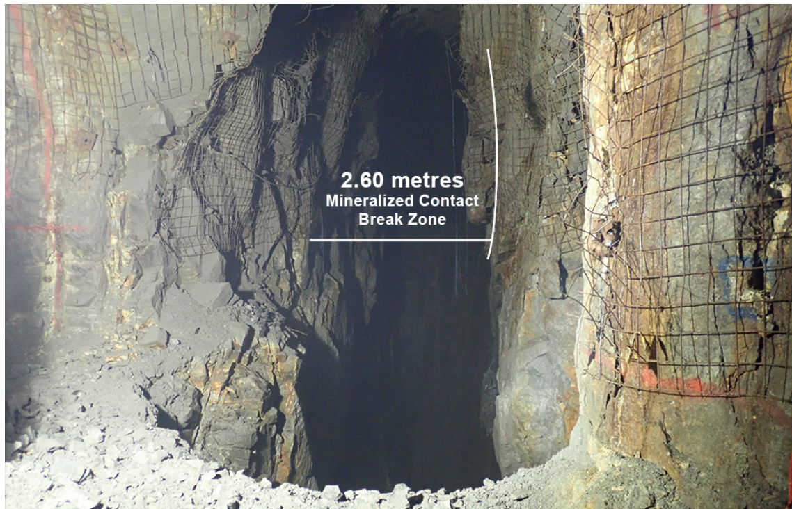
Figure 2: Photo of Stacked Trial Stope Demonstrating Excellent Blast Control and Clean Breakage Along the Mineralized Contact
