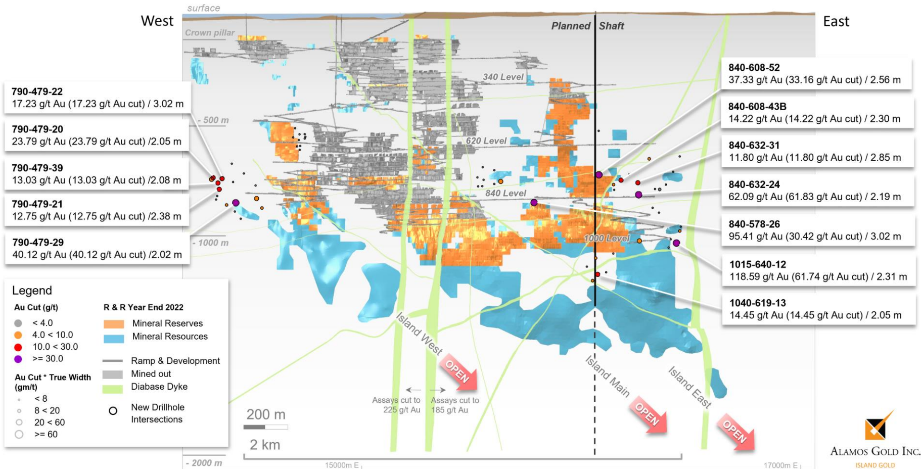
Figure 1: Island Gold Mine – C/E1E/E1EN/E1D Longitudinal, New C and E1E-Zone Underground Exploration Drilling Results
