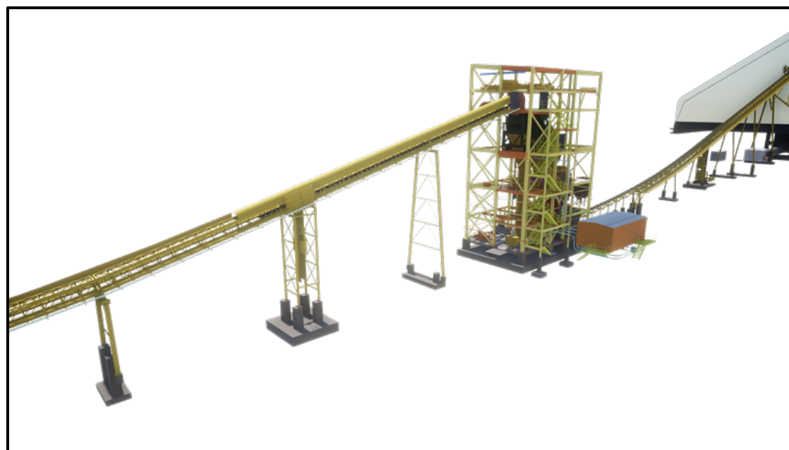
Figure 17-4 Secondary Crushing Installation
