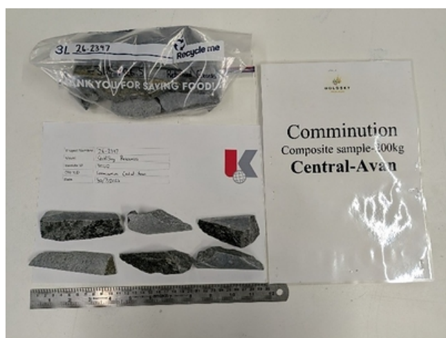
Image 2 : Sample preparation for Central and Avan zones of the Barsele Deposit
