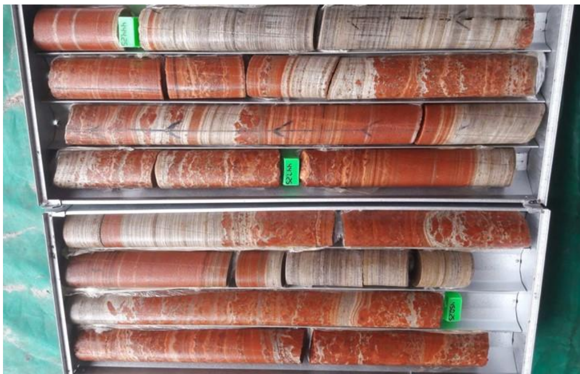
Figure 7.11: Drill Hole Ba-002 Core, Cycle VI Showing Banded Rock Salt with Carnallite Growth at the Layers Rich in Insoluble Material combined with more massive Carnallite, Resulting in a Carnallite Dominated Rock with Rock Salt
