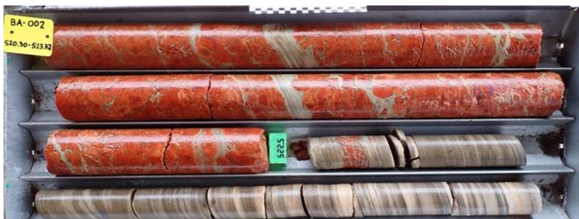
Figure 7.12: Drill Hole Ba-002 (extension) Core, Cycle IV Showing thick Layers Dominated by Nodular Carnallite, Separated by an Interlayering of Rock Salt and Insoluble Material
