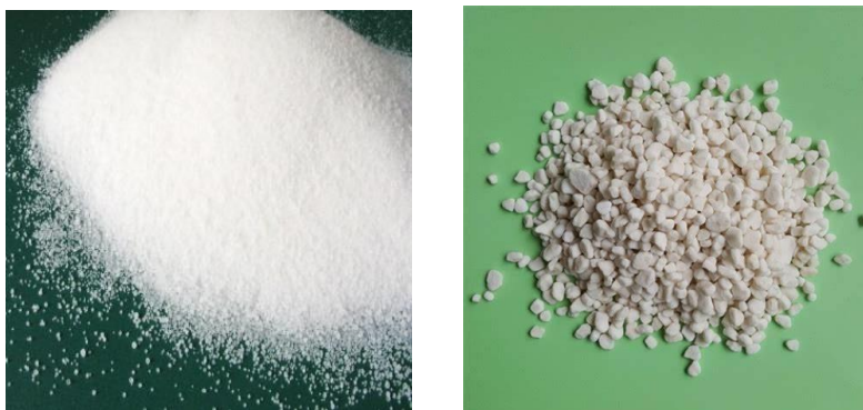
Figure 17.7: Recrystallised (white) Standard Potash (left) Compacted Granular MOP (right)
