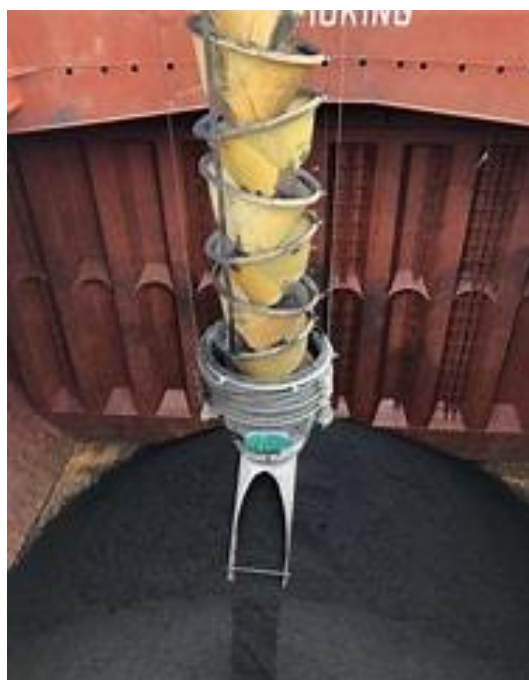
Figure 17.8: Cleveland Cascades Chute Loading from an Overhead Conveyor into a Ship Hold
