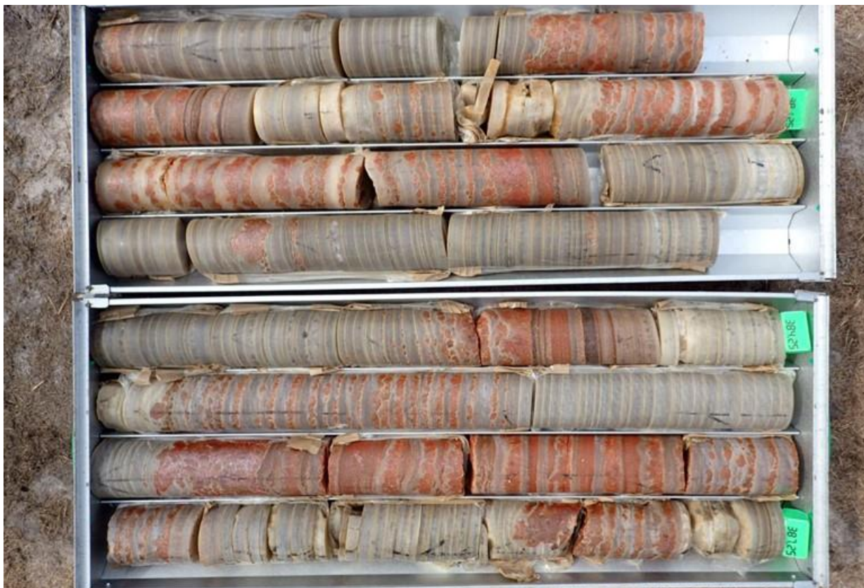
Figure 7.10: Drill Hole Ba-002 Core, Cycle VII Showing Banded Rock Salt with Carnallite Growth at the Layers Rich in Insoluble Material, Resulting in an Irregular Carnallite Rock Salt Interlayering
