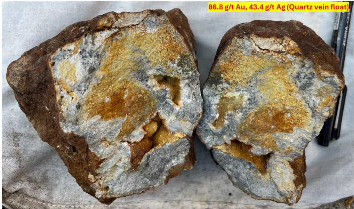
Figure 6 High grade quartz vein float, competent, open spaced cavities with strong silica/qtz-pyrite-clay. Fine-grained disseminated and clustered pyrite.
