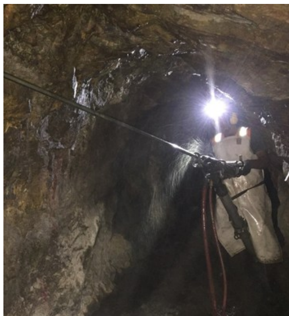
Figure 4: Drilling blast holes to expand underground tunnel (T-001) at San Marcial (CNW Group/GR Silver Mining Ltd.)
