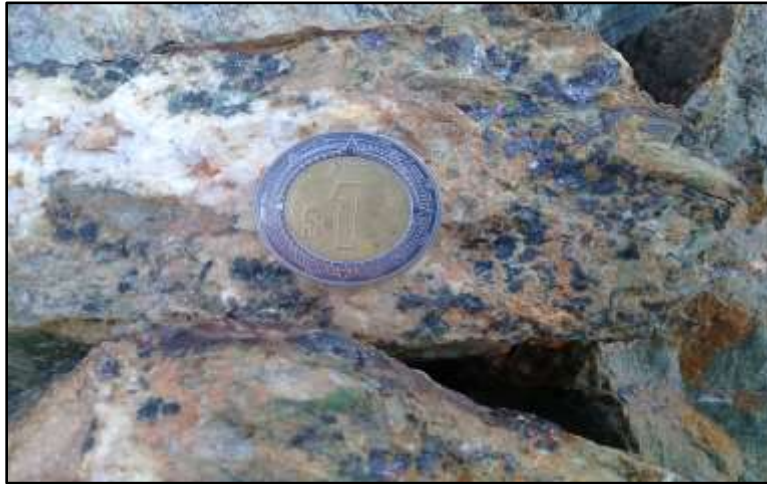
Bornite-chalcopyrite primary mineralization associated with stringer-type footwall carbonate veining in volcanics; sample from between highway and intrusive complex.
