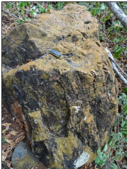
Figure 4. Photograph of a cylindrical block of 'gossan' interpreted to be a remnant conduit of hydrothermal fluids or 'black smoker'; note pocket knife for scale. (CNW Group/Vortex Metals)
