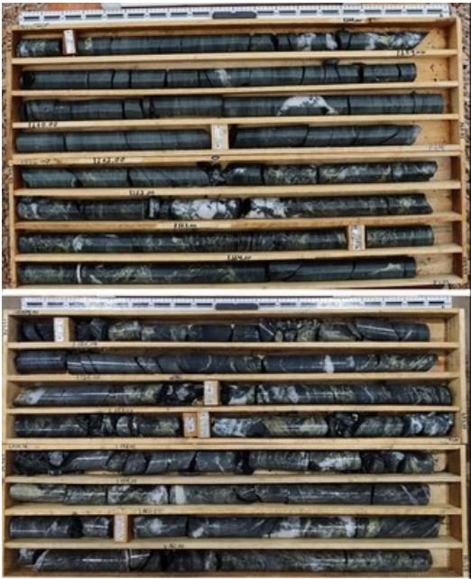
Photo 2 top: CD-003: Southern Copper Zone, Trays 47-48; 157.27 - 164.40m. Zone of stringer sulphides and quartz veining approaching sulphide breccia zone. Photo 2 bottom: CD-004: Southern Copper Zone, Trays 45-56; 153.96 - 161.68m. Zone of sulphide breccia and quartz veining. (CNW Group/Meridian Mining S.E.)
