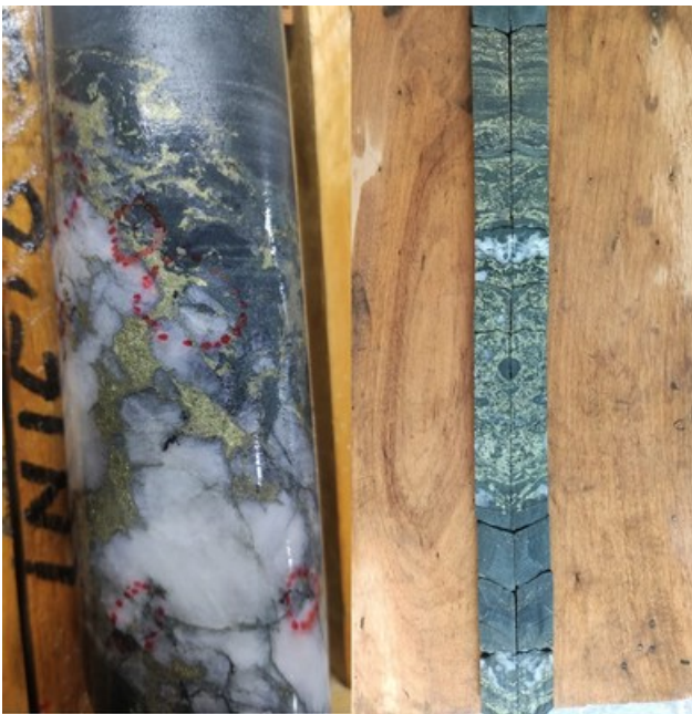
Photo 1: Left: CD-072: one of the high-grade Gold veins encountered with multiple points of visible Gold circled in red; Right: CD-070: chalcopyrite-dominant mineralization associated with strong chloritic alteration, interpreted to reflect proximity to a VMS feeder system. (CNW Group/Meridian Mining UK Societas)
