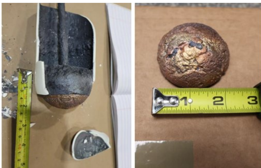
Photo 1: 300g copper blister sample produced from Cabaçal's copper sulphide concentrates
