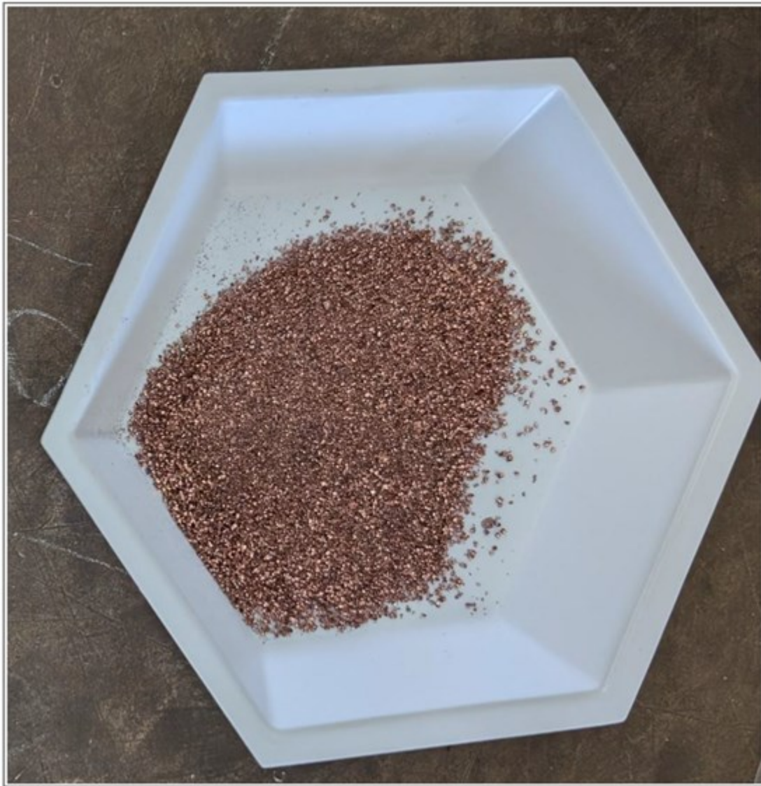
Photo 2: Copper sawings from high quality copper blister sample produced from Cabaçal's copper concentrates.
