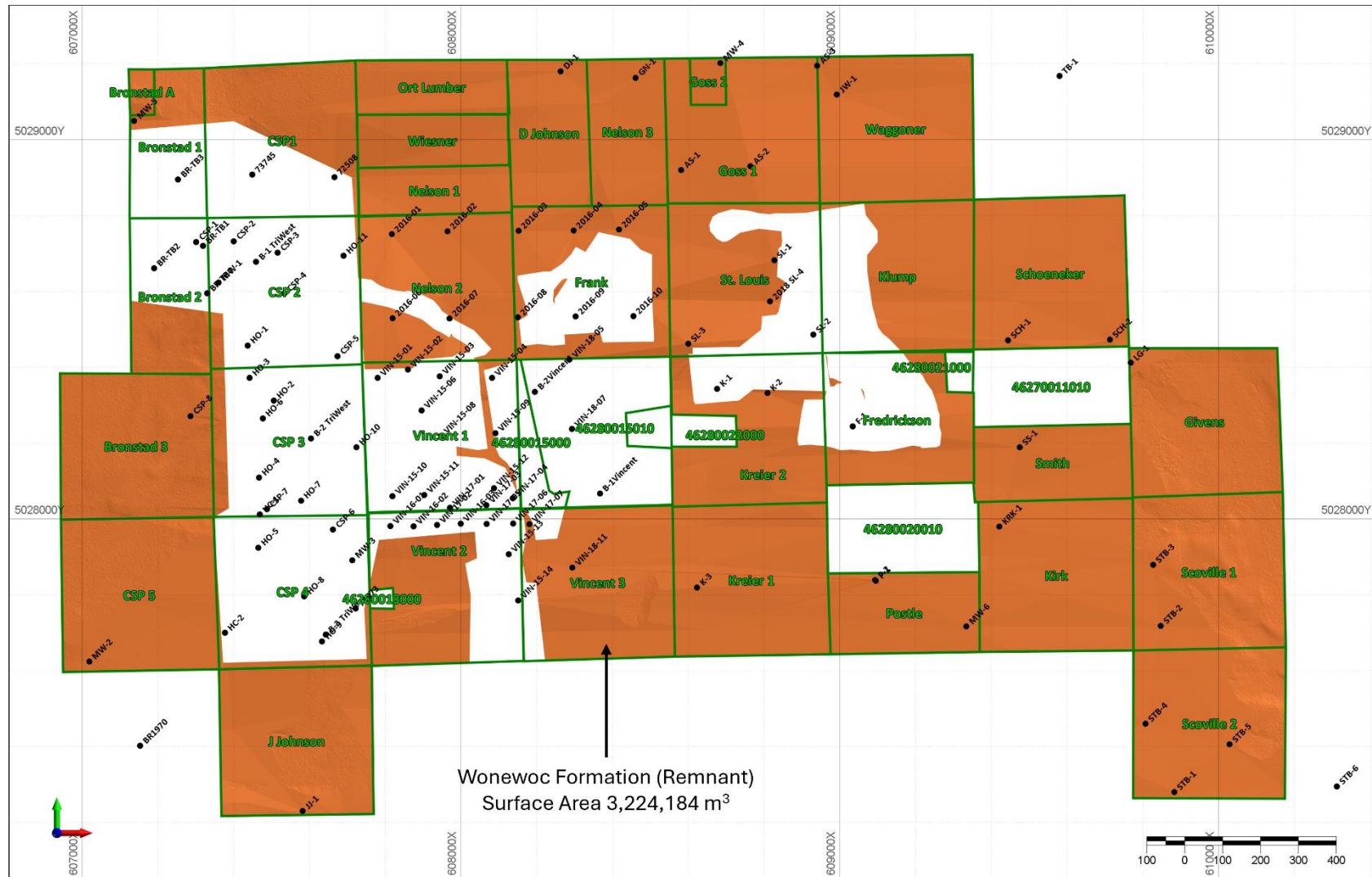
Figure 14.3. Plan view showing the Wonewoc Formation surface area used in the 2025 resource estimations. Blank areas show either mined out (Wonewoc depleted areas) or private property owner areas. Source Energy Services auger drillholes and the individual parcels also shown.
