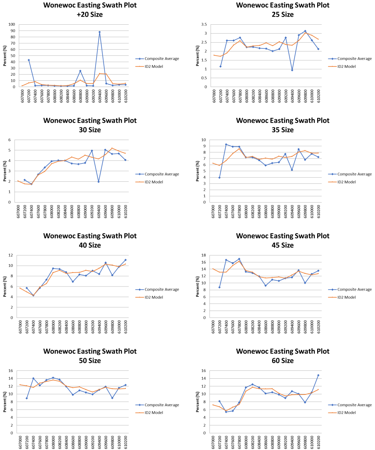
Figure 14.11. Easting SWATH plot of composite sizing (%) versus estimate sizing (%) in the block model.
