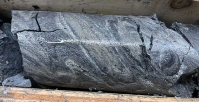
Photo 2: Grey Facies mineralization in TS25-003 laminated sphalerite and barite at 1,208.7 m (CNW Group/Fireweed Metals Corp.)
