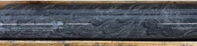
Photo 1: Selected interval of Black Facies mineralization in TS25-003 laminated sphalerite, barite, and mudstone at 1,198 m. (CNW Group/Fireweed Metals Corp.)
