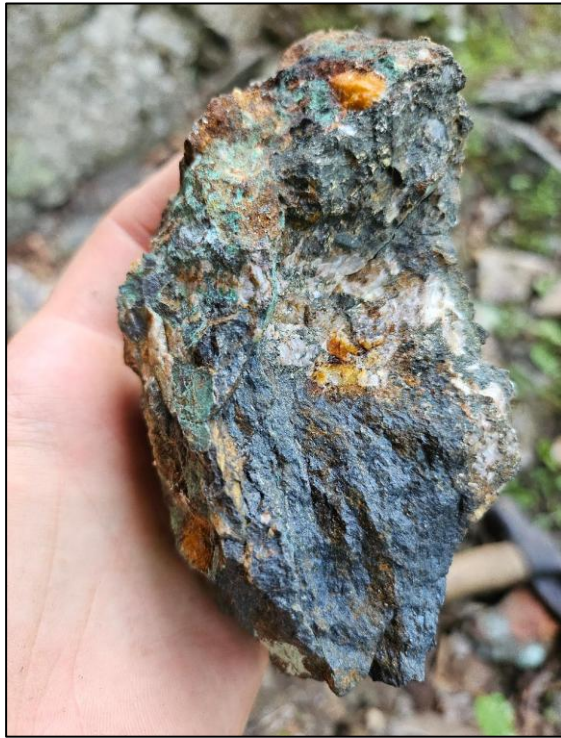
Figure 2: Maimann Lake area grab samples showing visible Chalcocite and Malachite
