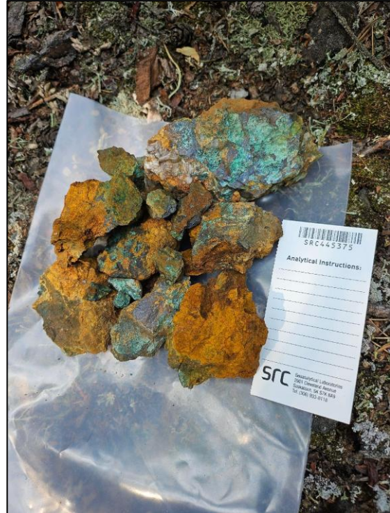
Figure 2: Maimann Lake area grab samples showing visible Chalcocite and Malachite
