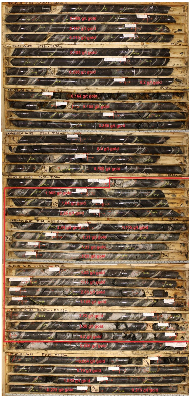
Photo 1 – Drill core from hole RY-25-01, 77.08 to 114.53 m annotated with individual sample results. Highlighted interval grades 1.98 g/t gold over 14.99 m.
