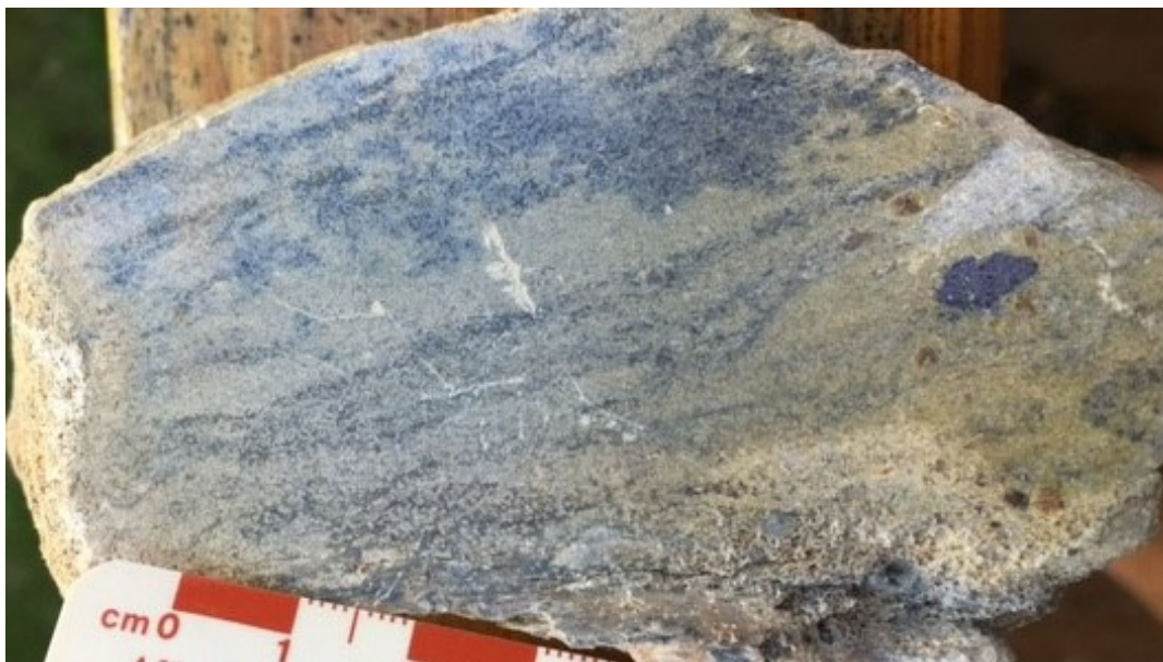
Figure 7-5 C-4 Sample - Yellow to honey coloured sphalerite, large galena and brown sphalerite blebs to the right, centimeter scale
