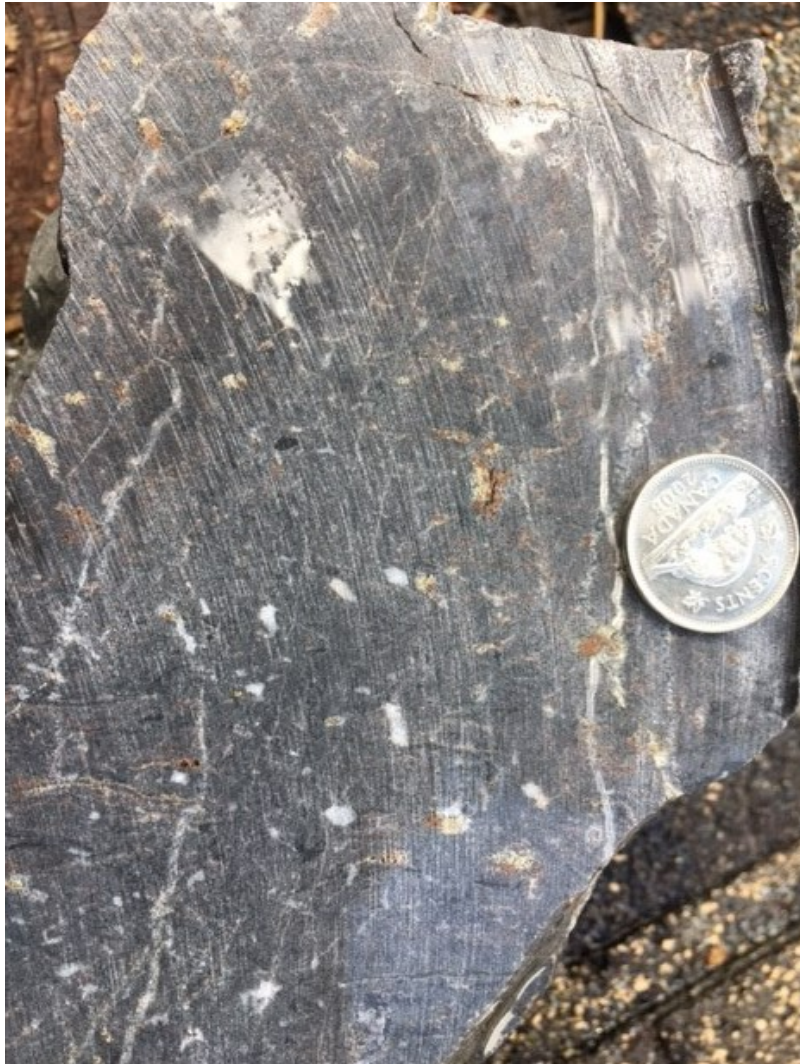
Figure 7-3 BMI Sample - Brown and red coloured sphalerite, birdseye texture, bedding dominated by fragmental material, prominent veining vertically, centimeter scale
