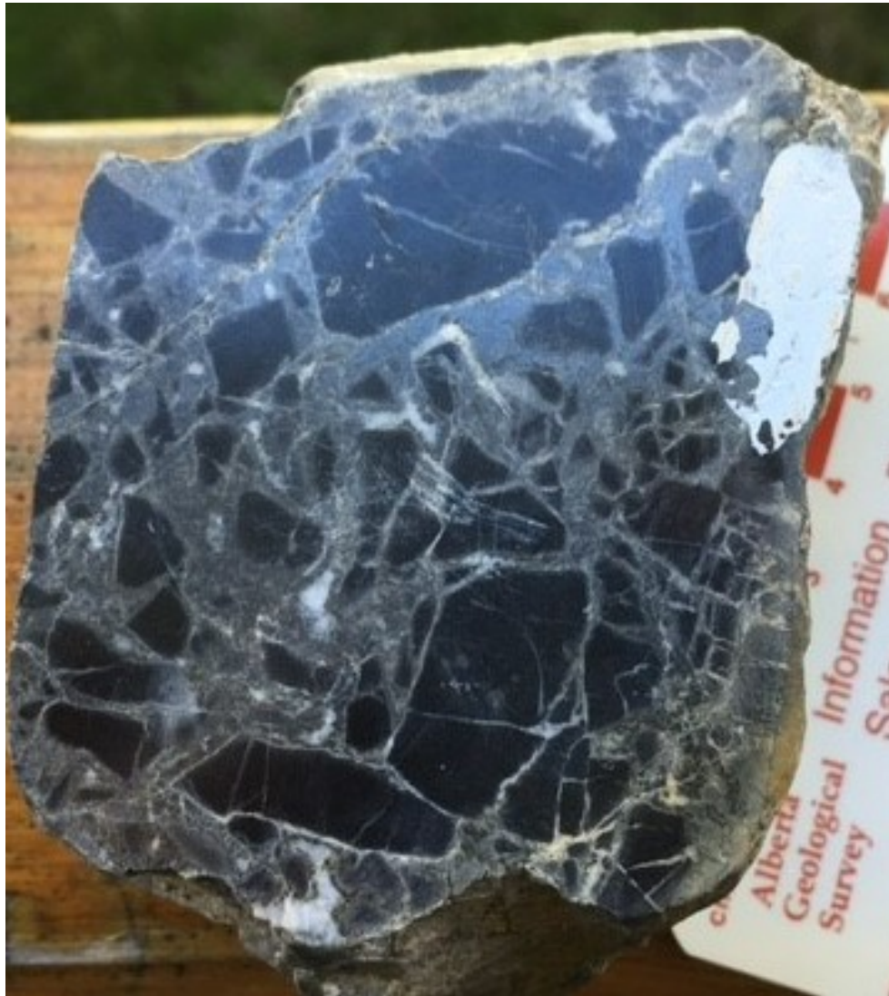
Figure 7-6 C-3 Sample - Yellow to grey coloured sphalerite as cement within the breccia, centimeter scale
