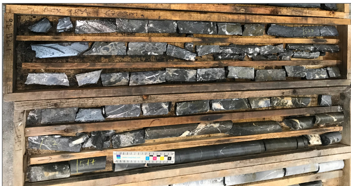
Figure 12.2 Drillhole 92-BL-1: Core trays showing interval 572.30 to 577.8 m, with high-grade interval 576.20 to 580.80 m (Zn = 4.48%, Pb = 0.73% and Ag = 6.18 g/t)
