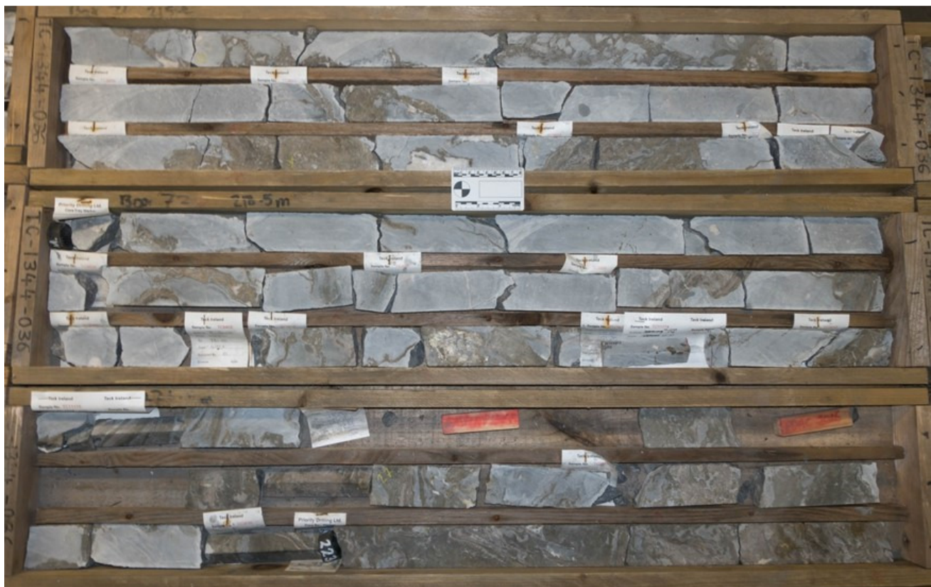
Figure 6.2 Core photographs showing semi-massive to massive sulphides, interpreted to display both open-space and breccia-replacement textures. Drillhole TC-1344-036 is in the north-central part of the Resource Estimate
