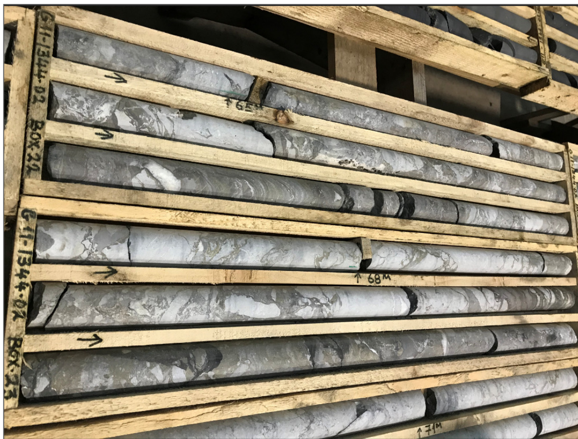
Figure 12.1 Drillhole G11-1344-02: Core trays showing interval ~64.8 to ~70.5 m, with mineralogical assemblage consisting of pyrite, sphalerite and minor galena
