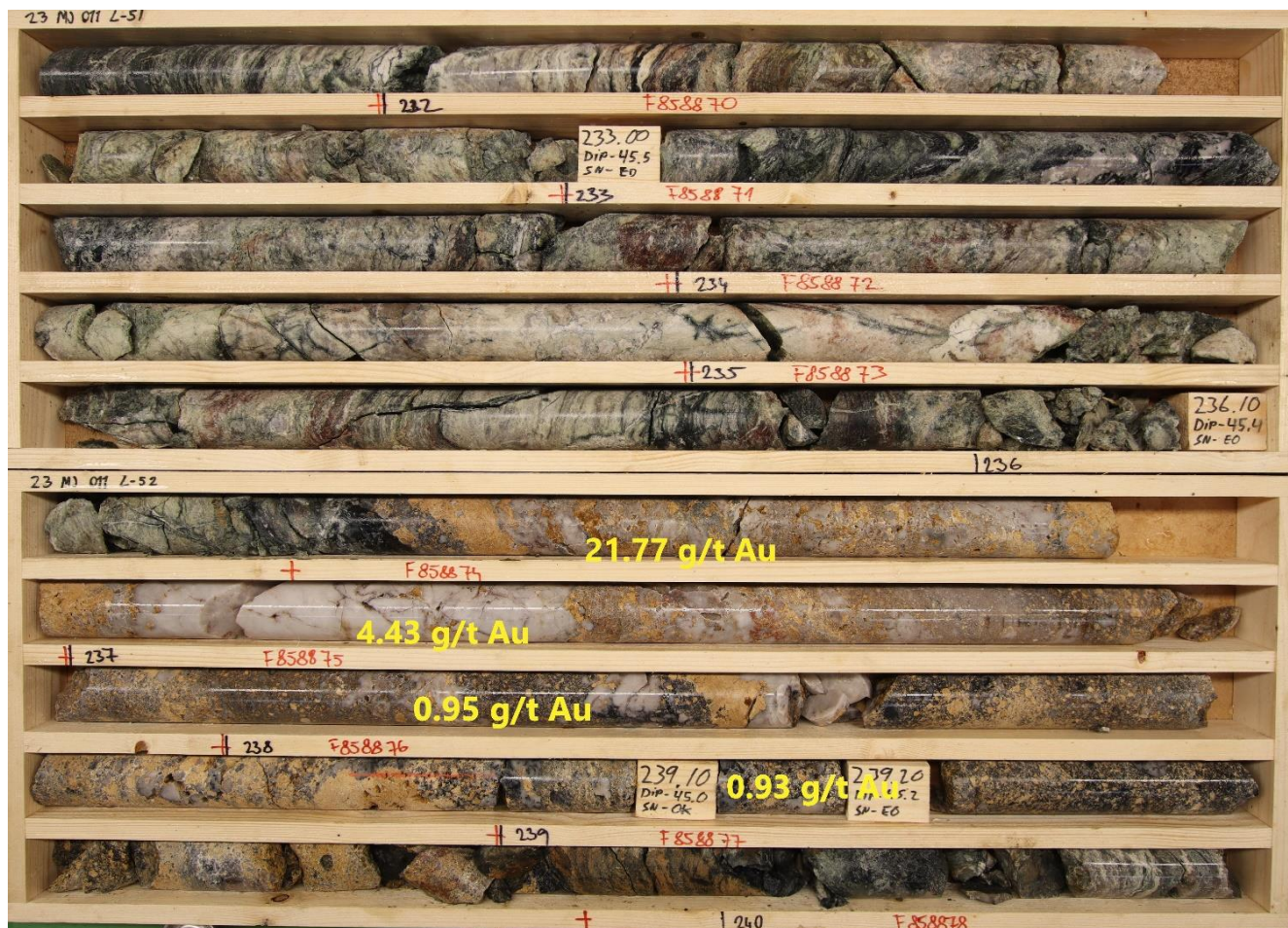
Figure 4. Fault breccia zone in 23MJ011 with 3.6m of 5.96 g/t Au from 236.3m downhole. Visible gold flakes were observed from two intervals grading 21.77 g/t Au and 4.43 g/t Au.
