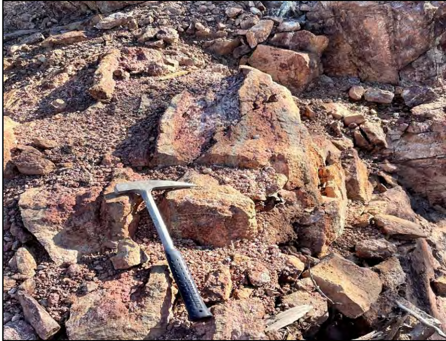
Figure 7-5. Northeast trending fractures, northeast target. The hammer is sub-parallel to the trend of the fracture, indicated by cream-colored argillic altered bands just above the hammer head. Sample 412778 (2.13% Cu) was collected just below this photo along the excavated face shown in Figure 7-6.
