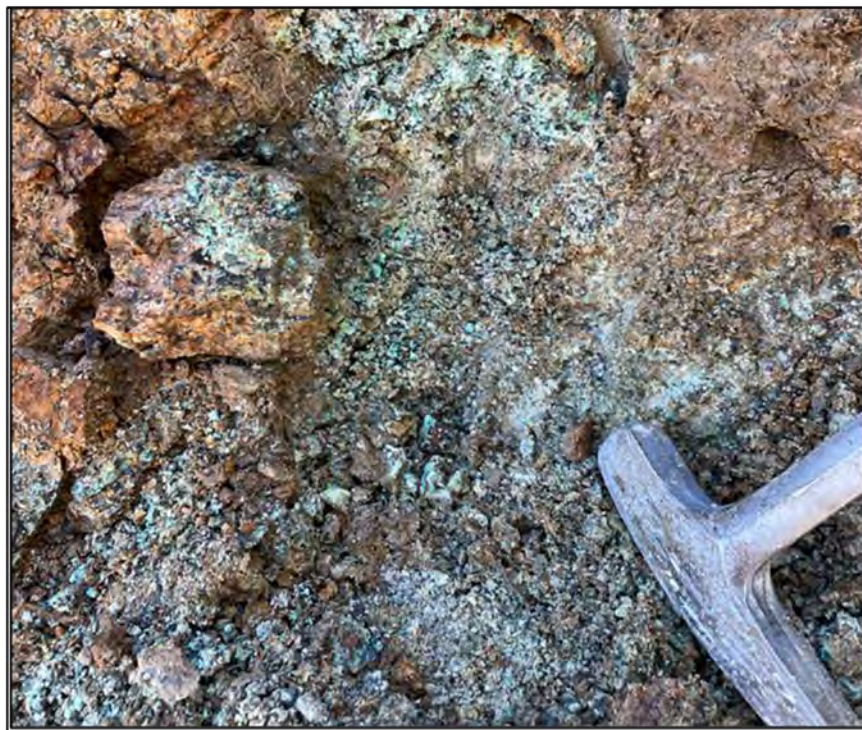
Figure 7-7. Disseminated chrysocolla in weathered, decomposed Precambrian granite. The sample# 412776, containing 1.34% Cu, was collected on the south wall of the small open pit near the center of section 18, T19S, R15W.
