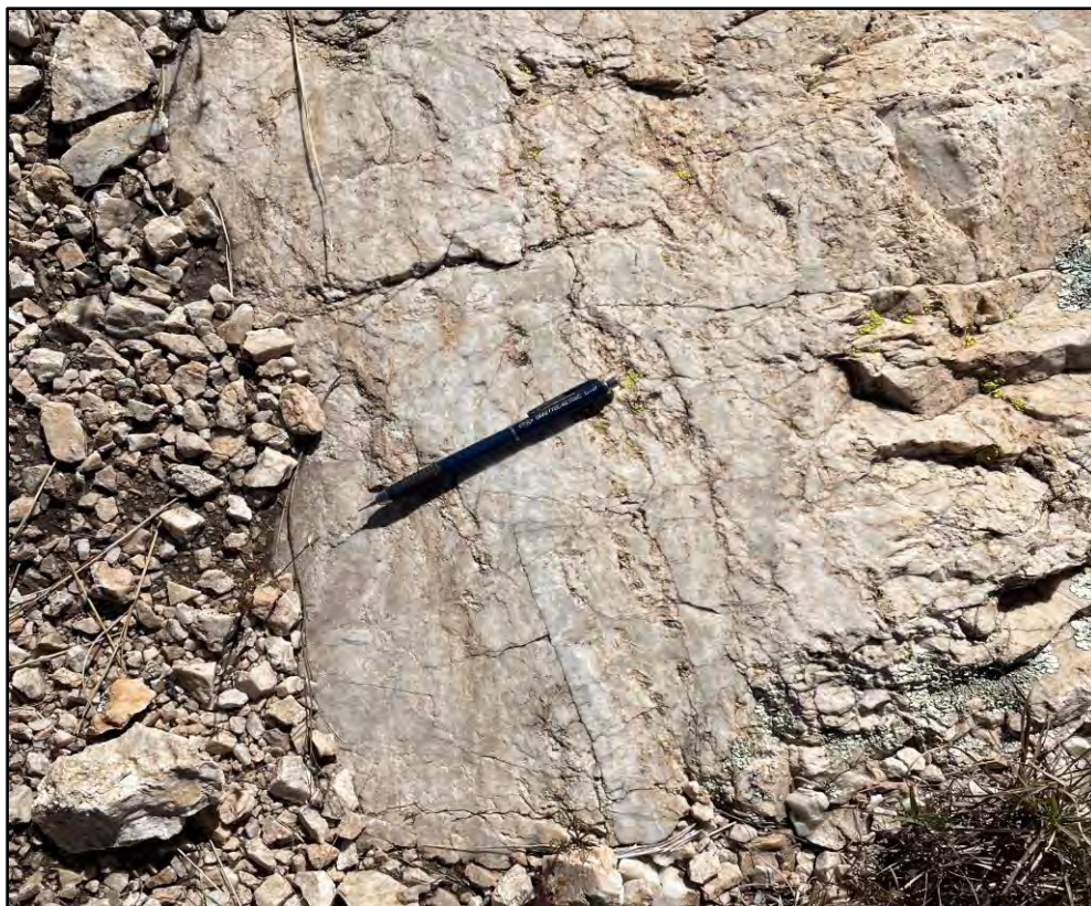
Figure 7-3. Strong pervasive replacement and stockwork veining in quartz monzonite(?). The photo was taken at the top of Sugarloaf hill.
