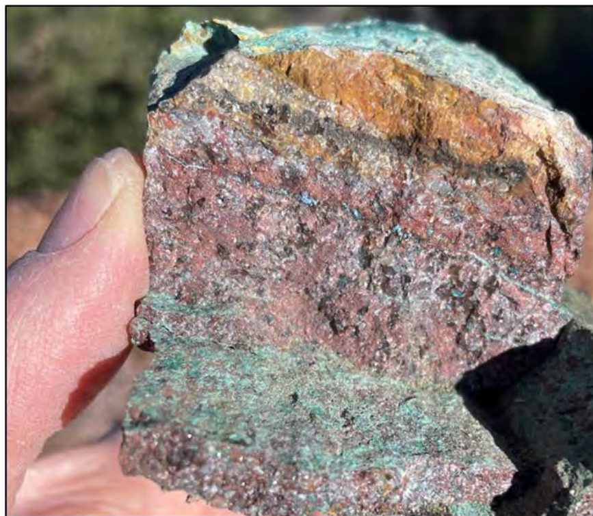
Figure 7-4. Chrysocolla and occasional malachite. Copper occurs as disseminations, along fine seams and along fracture surfaces. Goethite and late quartz veinlets occur at the top of the photo. Sample #412779 assayed 1.41%Cu.
