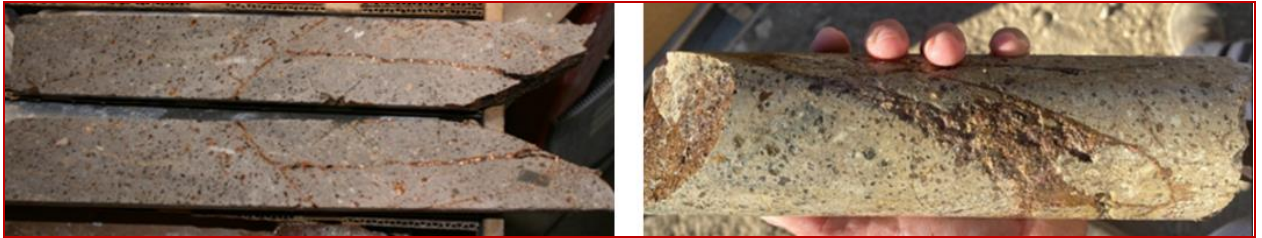
Figure 4: MHB-9:980 ft (298.6 meters) Native Copper
