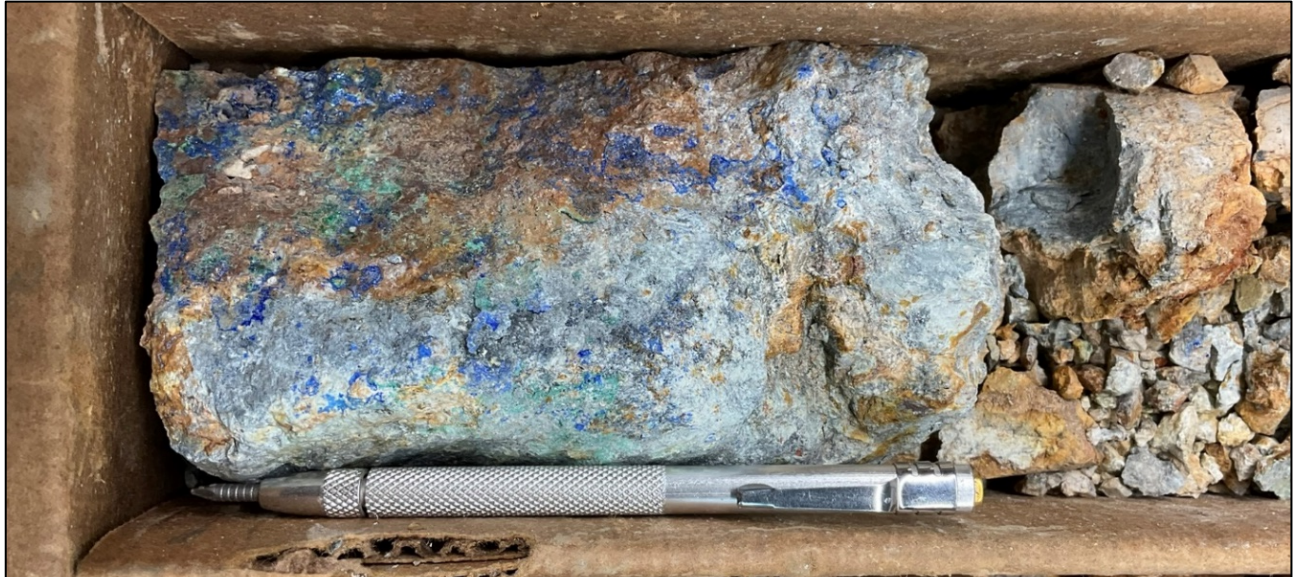
Figure 3: MHB-30 55.5-57.0 meters (182-187 ft /4.5% Cu & 49.0 g/t Ag with Strong Copper Oxides in Mineralized Breccia
