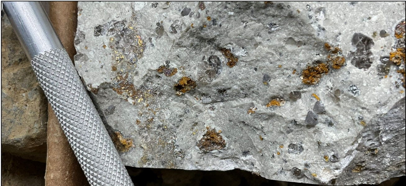
Figure 4: MHB-30 47.9-49.4 meters (157-162 ft)/2.1% Cu & 16.3 g/t Ag in Mineralized Breccia fragment with chalcopyrite and bornite
