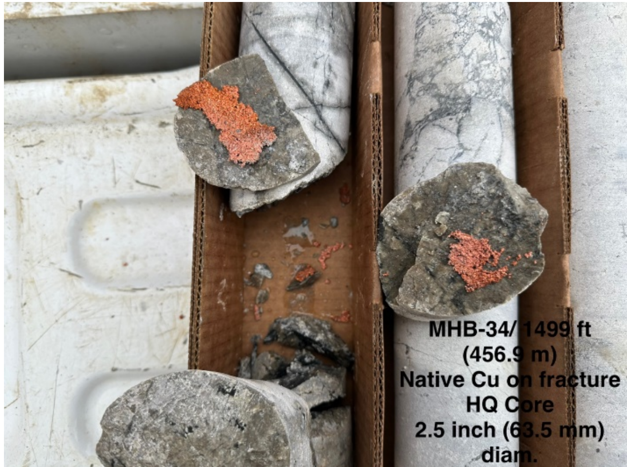
Figure 1: MHB-34/1499 ft (456.9 m) Native Cu on fracture HQ Core, 2.5-inch (63.5 mm) diam.
