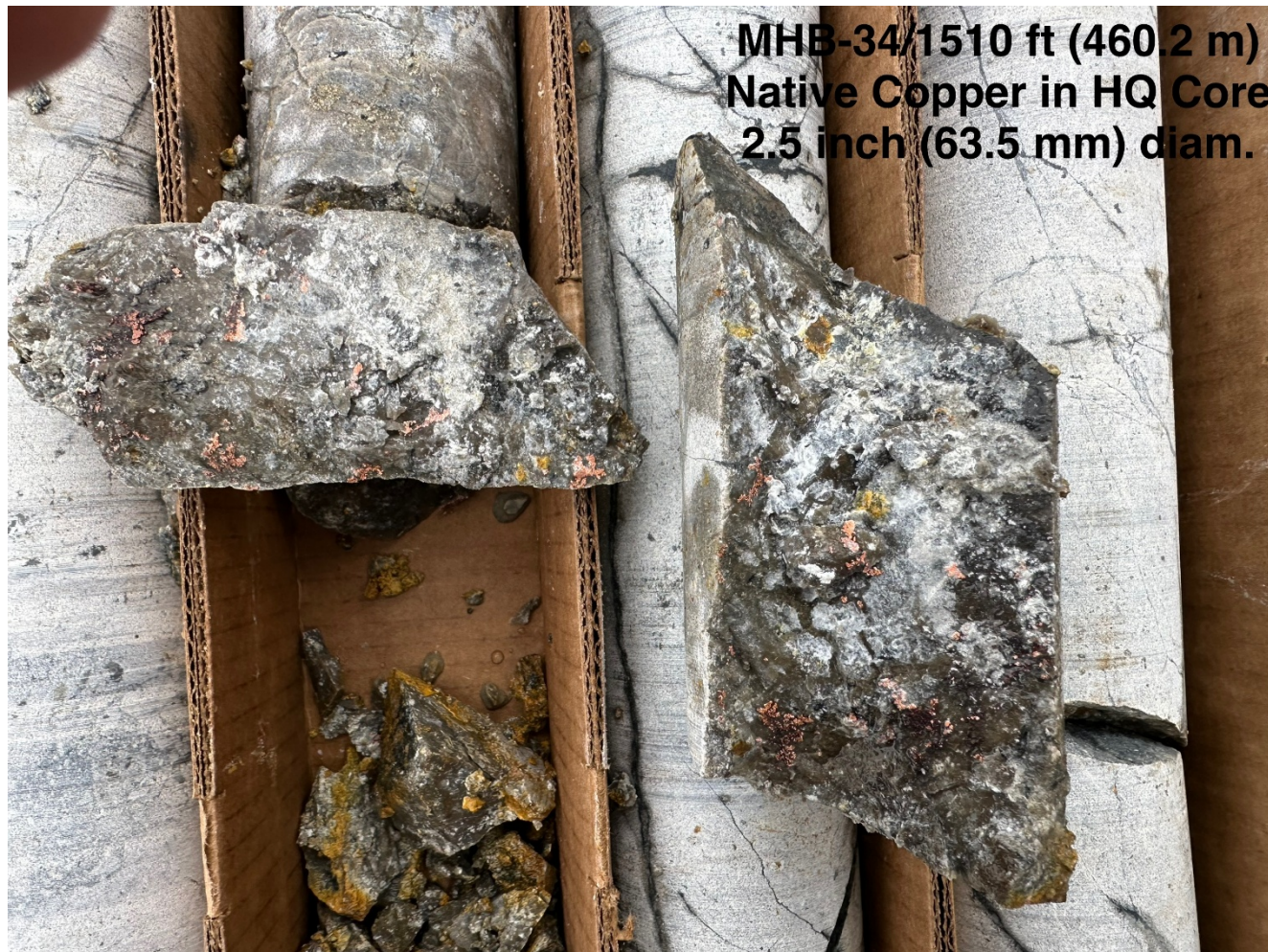
Figure 2: MHB-34/1510 ft (460.2 m) Native Cu in HQ Core with chalcopyrite, 2.5-inch (63.5 mm) diam.
