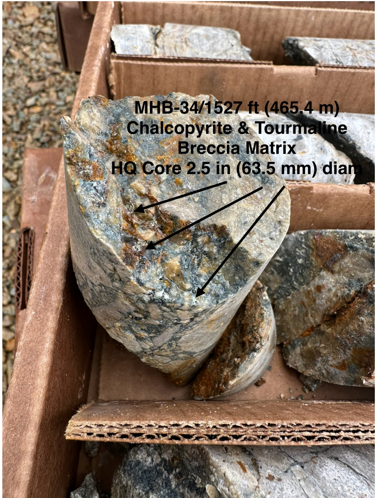
Figure 3: MHB-34 1527 ft (465.4 m) Chalcopyrite and Tourmaline Breccia Matrix, HQ Core 2.5-inch (63.5 mm) diam.
