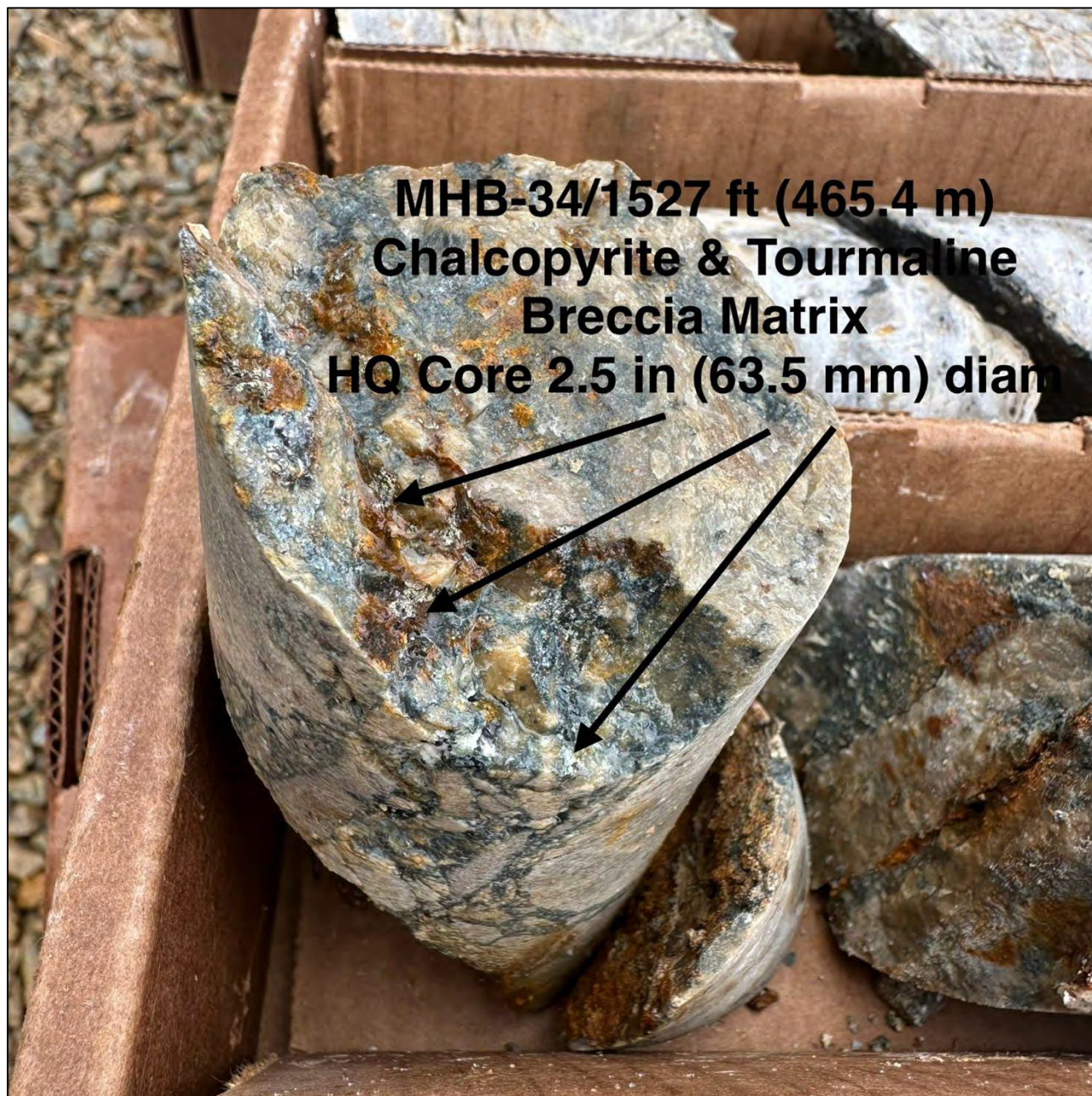
Figure 5: MHB-34 1527 ft (465.4 m) Chalcopyrite and Tourmaline Breccia Matrix, HQ Core 2.5-inch (63.5 mm) diam.
