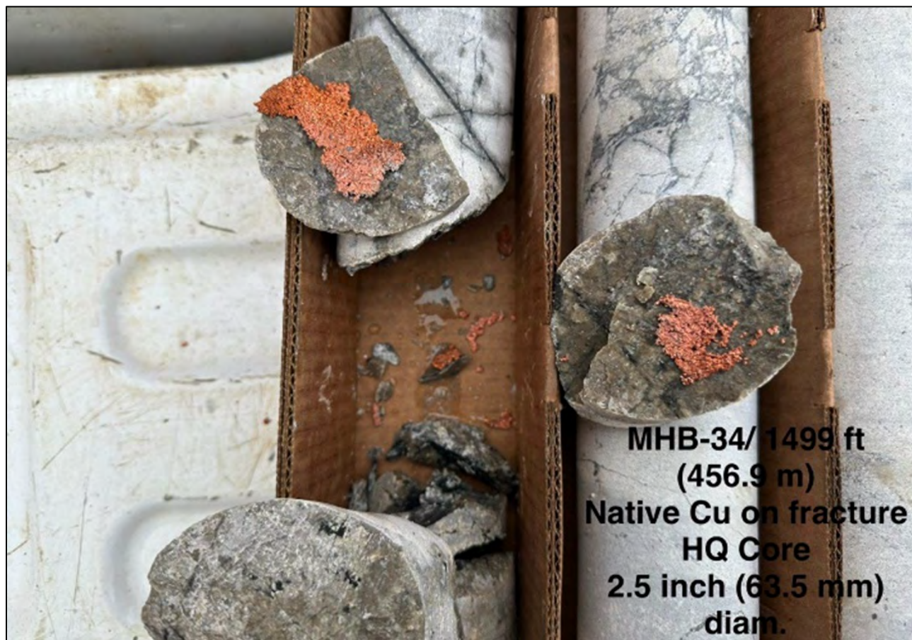
Figure 3: MHB-34/1499 ft (456.9 m) Native Cu on fracture HQ Core, 2.5-inch (63.5 mm) diam.
