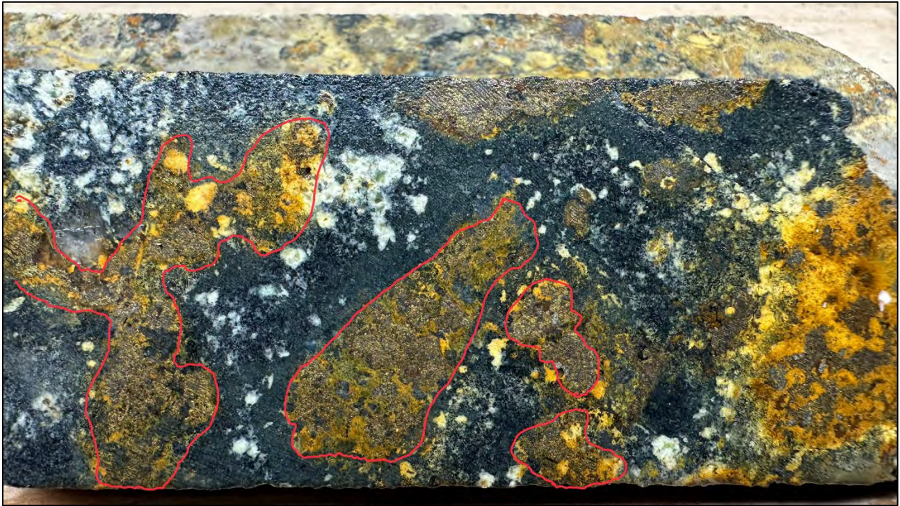
Figure 2: MHB-32 NQ Core closeup. Clasts of intrusive with chalcopyrite in tourmaline/chalcopyrite matrix breccia at 810 ft (246.89 m).
