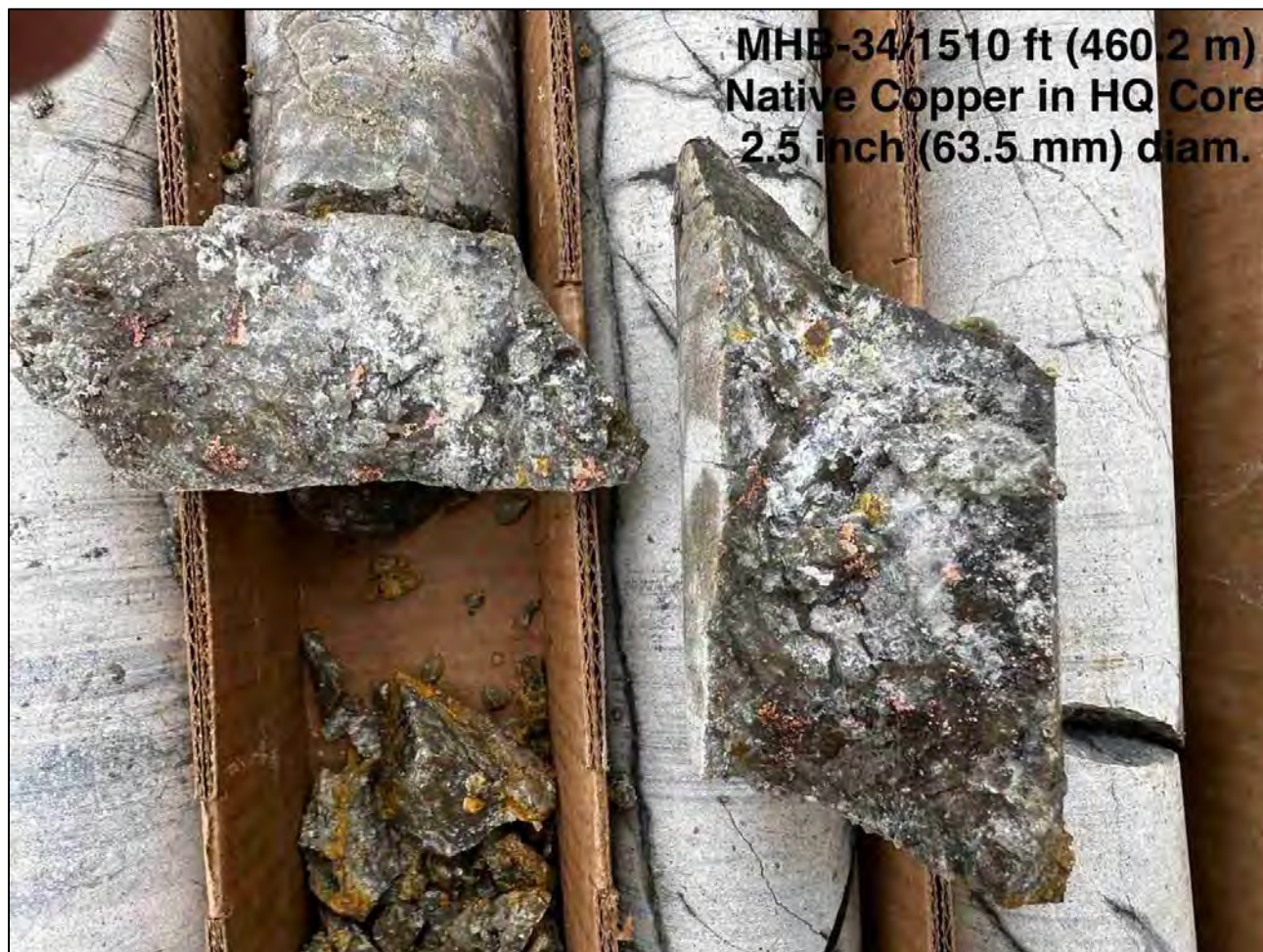
Figure 4: MHB-34/1510 ft (460.2 m) Native Cu in HQ Core with chalcopyrite, 2.5-inch (63.5 mm) diam.
