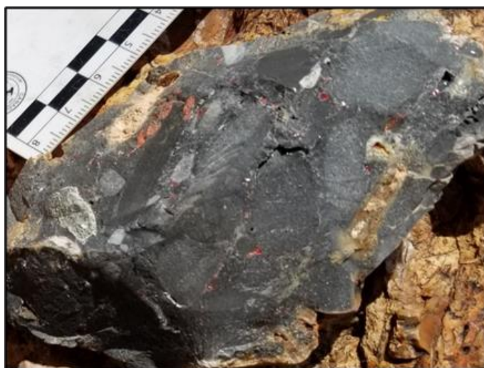
Centauro Gold Project: Blebby to semi-massive realgar and orpiment in siliceous breccia (0.042 g Au/t; surface grab sample 796497).
