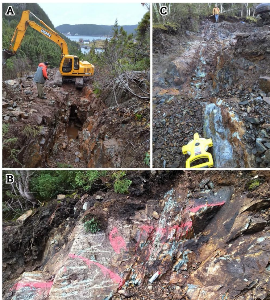
Figure 1 – a) Historical Stewart Shaft Exposed b) Polymetallic Central Vein at Taylor's Room c) New Discovery Polymetallic Vein at Pomley Cove Pond (one of four trenced)
