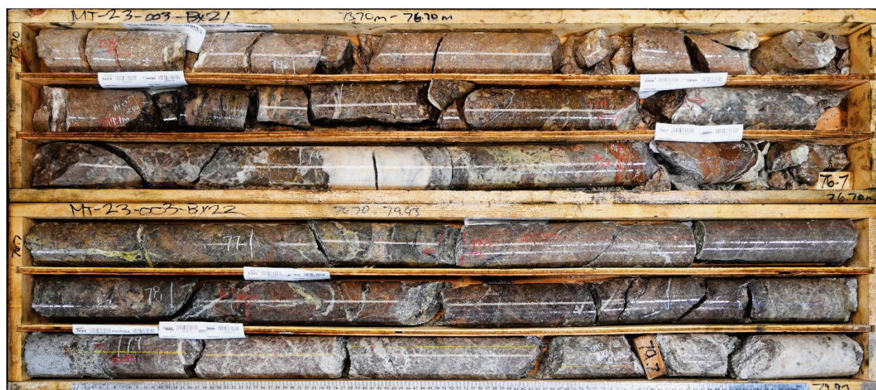
Image 1. MT23-003; mineralization grading 8.95 g/t Au and 2 g/t Ag over 9.2 m at 71.0 m depth (metal ruler is 1.0 m total length).
