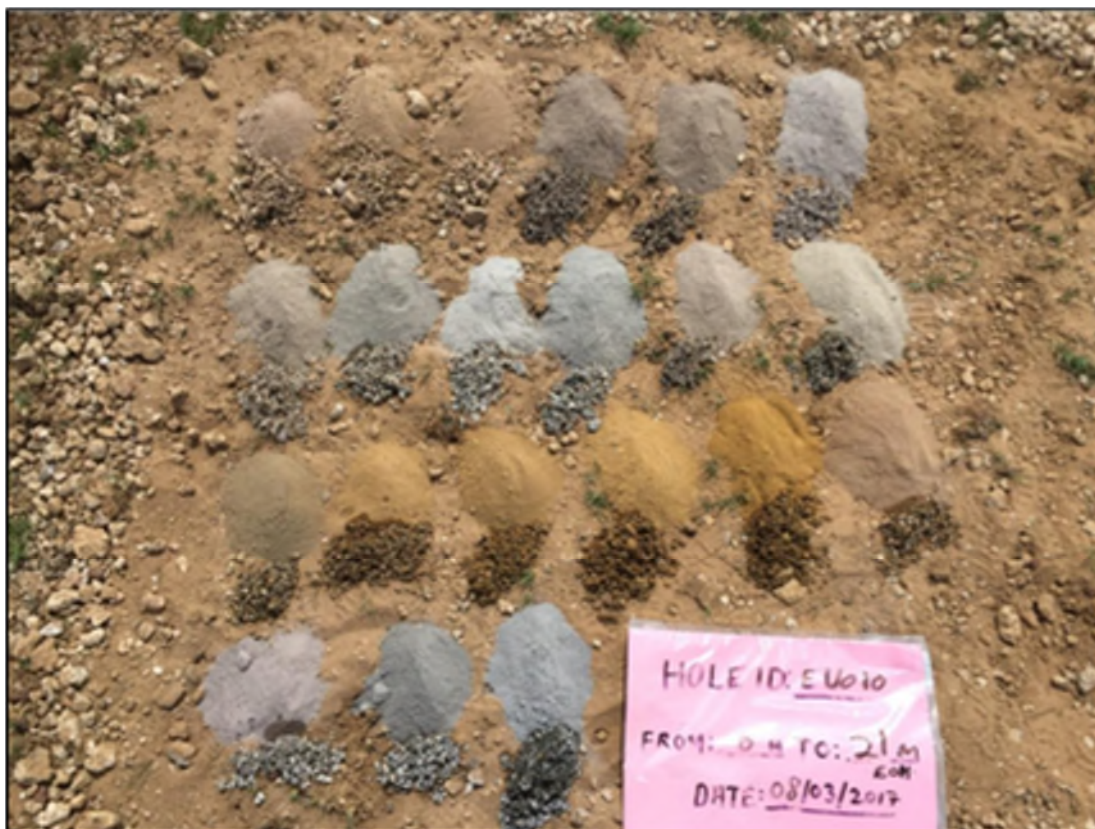
Figure H: RC chip pad showing the dust and chips for each metre drilled. The third row demarcates carbonatite samples.
