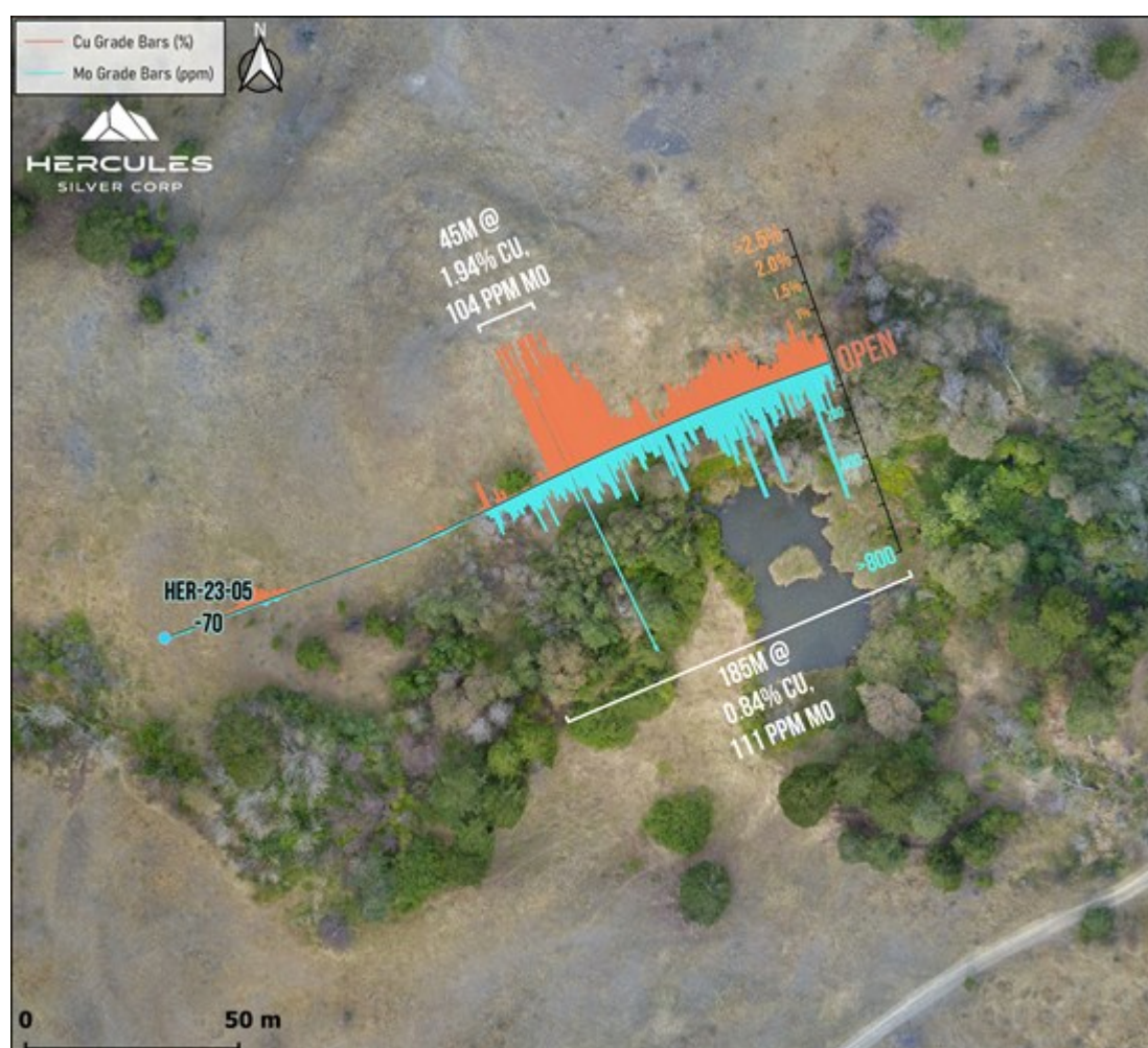
Figure 1: Plan view of discovery hole HER-23-05, collared in the Frogpond Zone showing grade bars for copper (orange) and molybdenum (blue).
