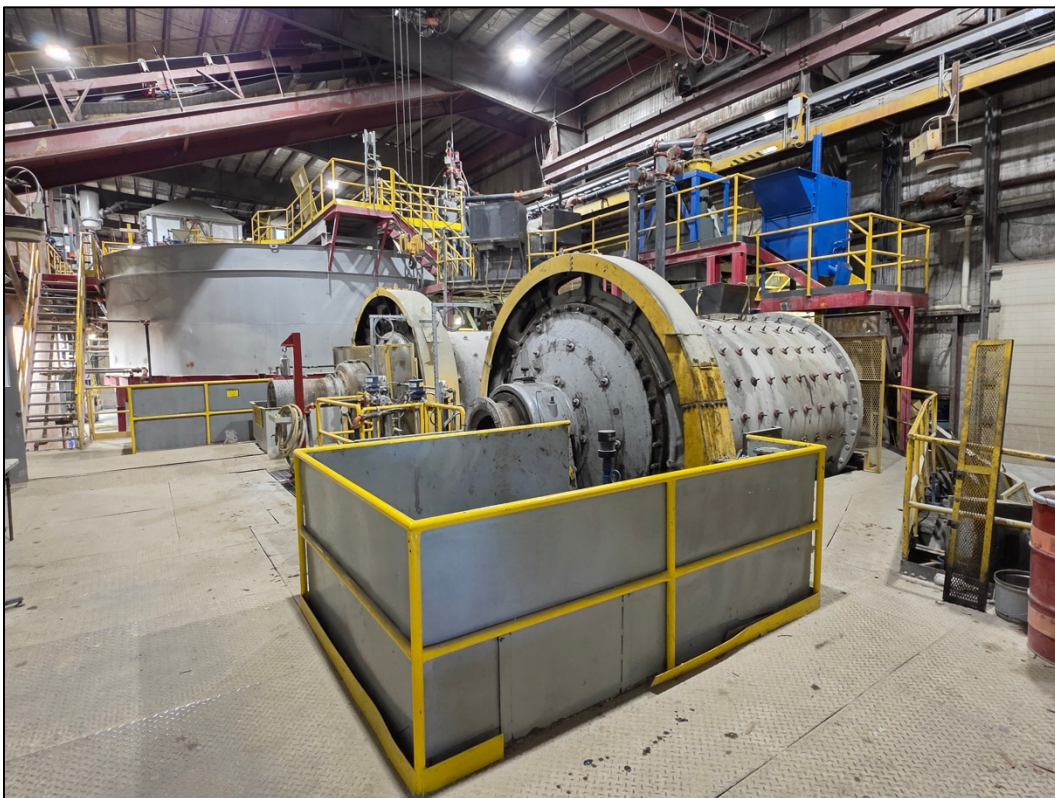
Photo 2: Ball and rod mills within grinding circuit
