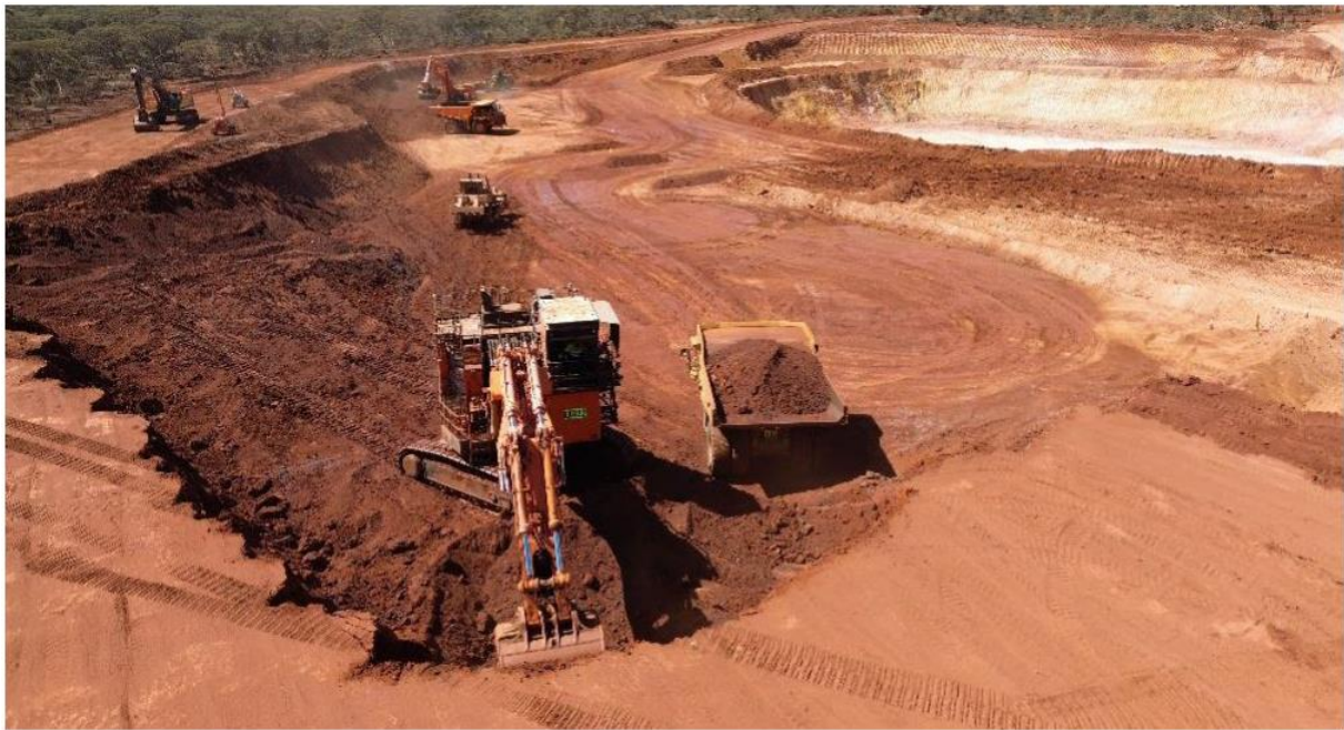
Figure 1: Myhree open pit 'free dig' mining, no requirement for drill & blast to date
