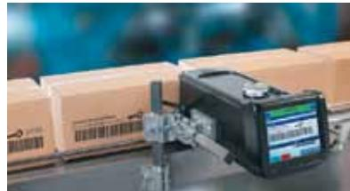
Xaar's extensive range of printheads allows for simple integration into a range of printing systems for coding and marking applications. These offer precise print capabilities directly onto carton board, replacing the need to pre-print cases or labels.
