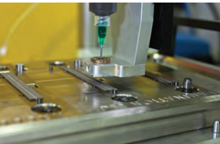
Xaar 1001 printhead manufacture During the lamination stage of manufacture, two key components are bonded – a uniquely numbered ceramic tile and PZT.
