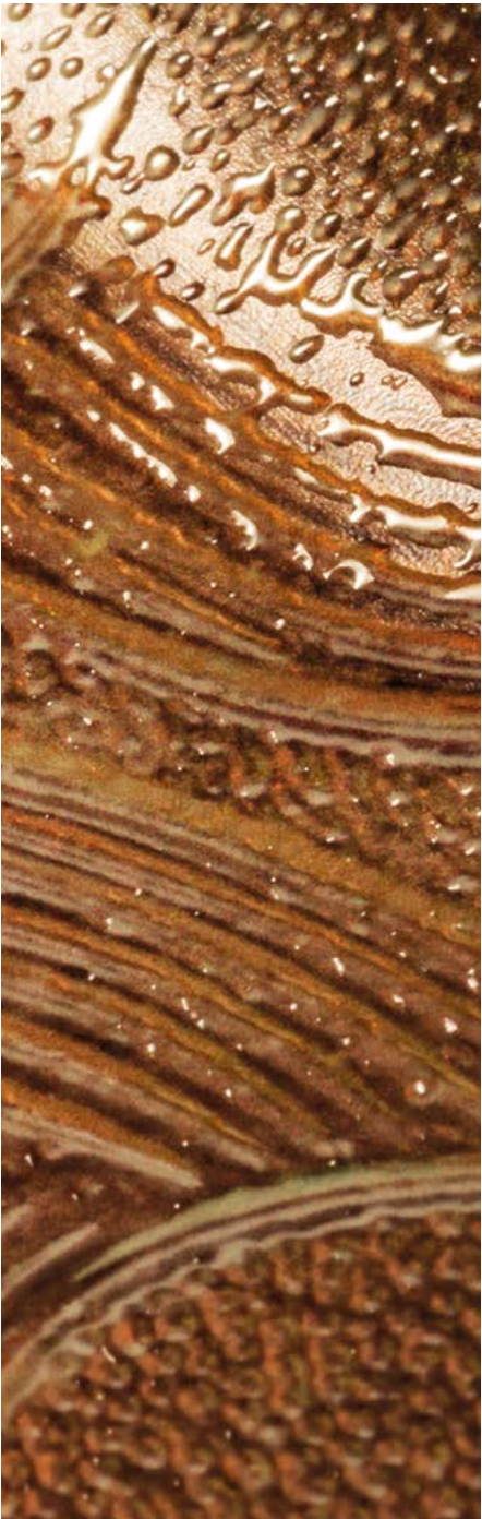
High Laydown Technology printed using Xaar 1003 printheads has been used to create tactile effects on labels
